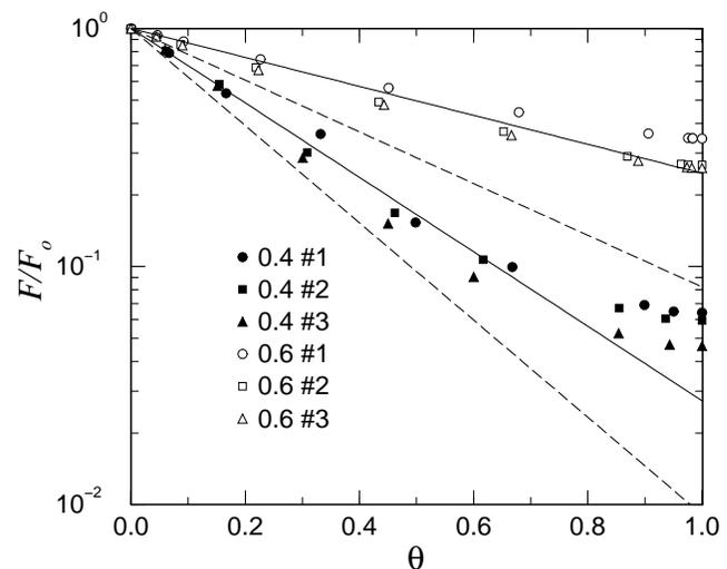
Figure 1: Relative change in the formation factor  $F$  as a function of the fraction  $\theta$  of calcium hydroxide that has been leached.
