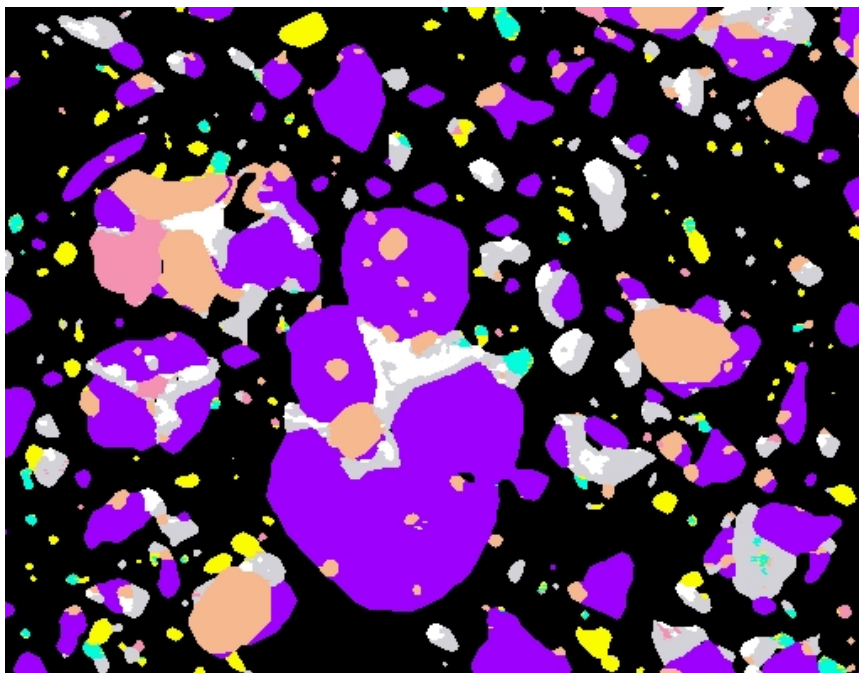
Fig. 4. Pseudo-colored scanning electron microscope image of portland cement shows the multi-phase character and particle shapes resulting from the grinding of clinker and gypsum with alite (purple), belite (tan), ferrite (white), aluminate (silver), periclase (pink), alkali sulfate (green), and gypsum (yellow). CCRL Cement 135, field width: 150 \mu\text{m} . Note: Colors shown only in online version.
