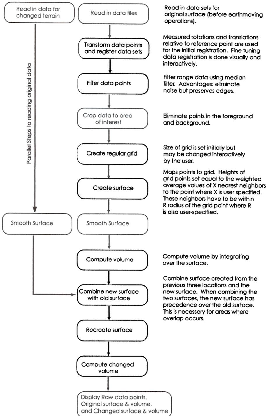
Fig. 6. Flow chart to display the LADAR data as point clouds and surfaces.
