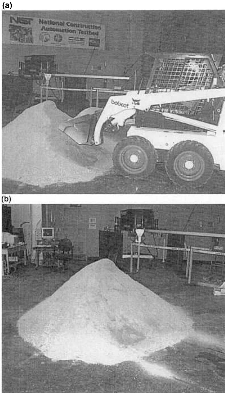
Fig. 10. (a) Modifying the pre-scanned scanned sand pile. (b) Photo showing the “changed terrain”. (c) Re-scan of the sand pile from one location (facing removed material). (d) Combine new scan with old scans from other three locations and regenerate 3-D surface. Color fringe contours denote depth of material removed. The total volume remaining, and the volume removed is listed.
