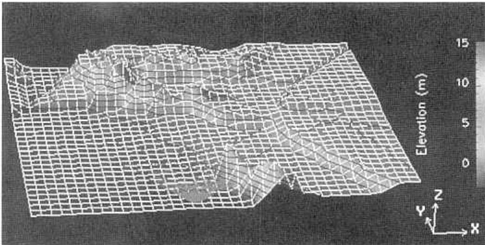
Fig. 3. Meshed surface of scanned terrain on NIST campus created using Data Explorer scripts.
