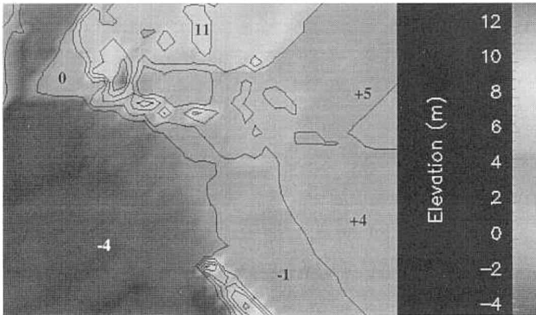
Fig. 4. Automatically generated cut/fill map created by operating on the 3-D terrain model of Fig. 3 with a final target elevation at  $z = 2$  m. Negative numbers represent fill requirements (in m) while positive contours represent cut requirements.
