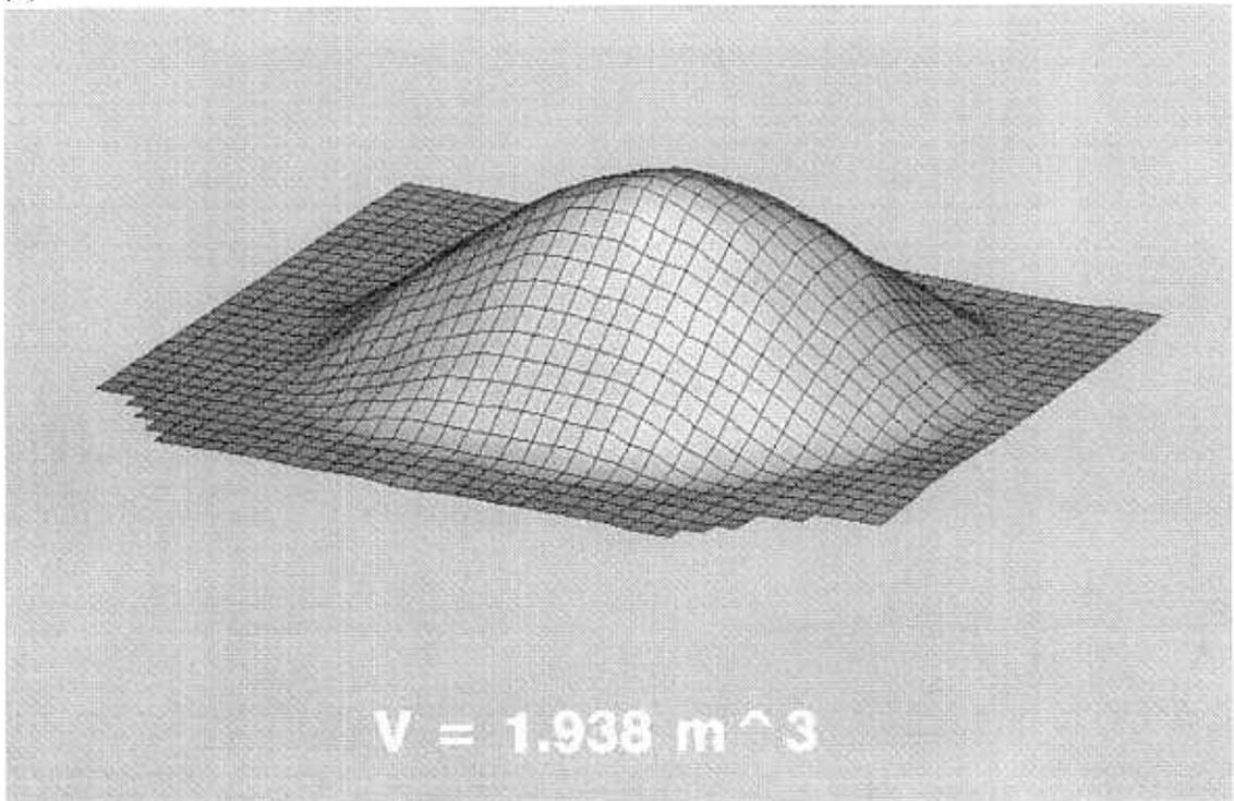
Fig. 9. 3-D surface of sand pile. (a) Combined point cloud from four scans. (b) 3-D surface.
