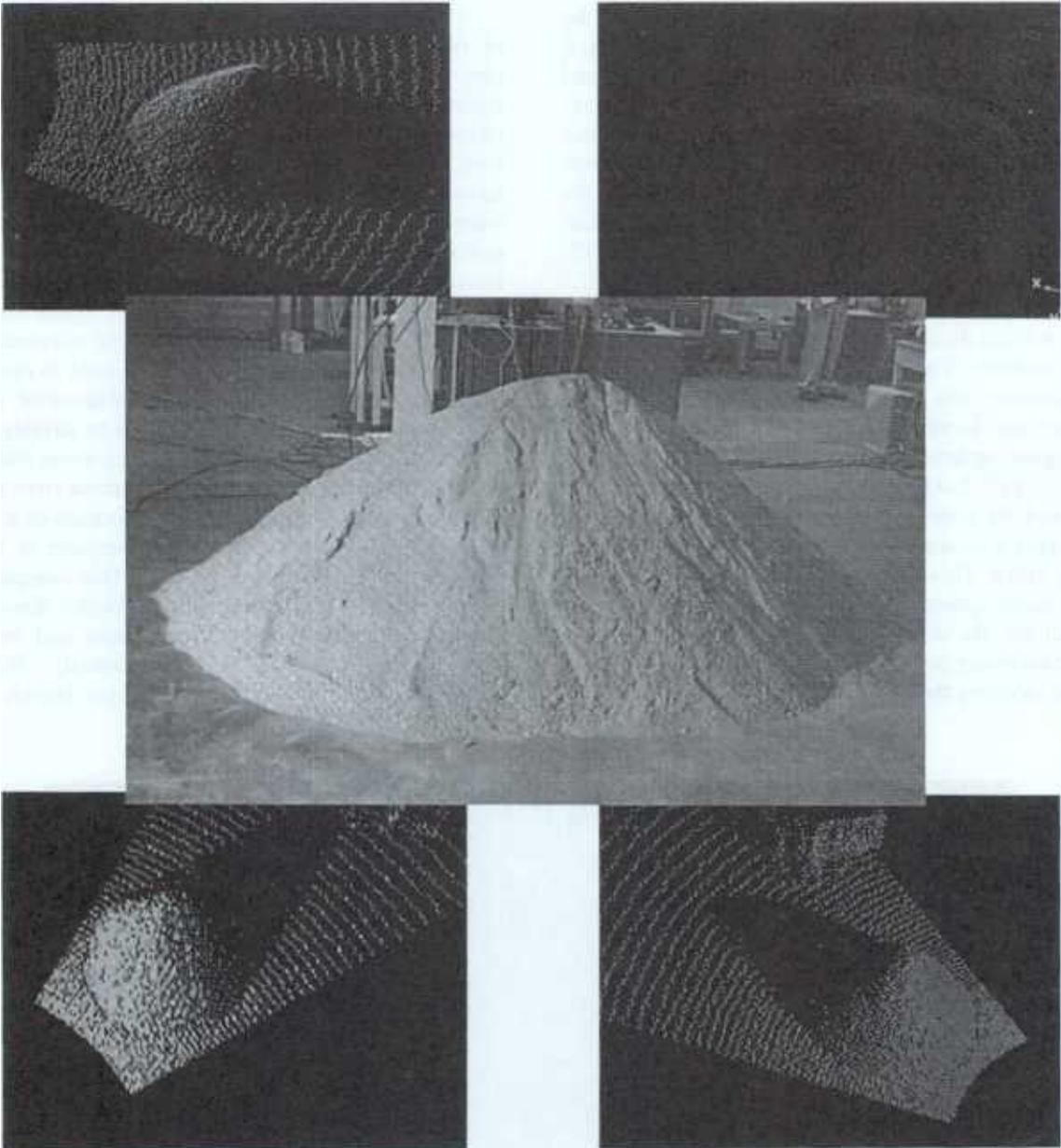
Fig. 5. Demo sand pile and the four point clouds obtained from the laser scanner.
