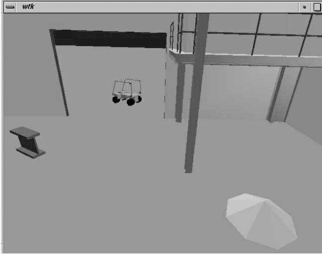
Figure 3g: “Live” visualization of the site. The field data collector acquires up-to-date locations for part fiducial points and makes these available the construction management system. A 6 DOF part localizer uses the data provided. It performs an optimization analysis to best locate the part origin and the yaw, pitch, and roll for the part. This derivative data is then made available to the temporal project database. Another automated agent, known as the VSS (for Virtual Site Simulator) is a 3D Augmented Simulation system that creates a data-driven three dimensional view of the construction site showing the current status of tracked components, scanned terrain data, and tracked machinery. The I-beam described in the previous figures is shown at left center, properly updated after being moved and re-measured. Updates are generally discrete, quantized changes, since measurements will typically only be taken at the conclusion of each move of the component. However, the NIST system can handle real-time update rates that permit live tracking of a component placement as well as the tracking of the machine manipulating the object.
