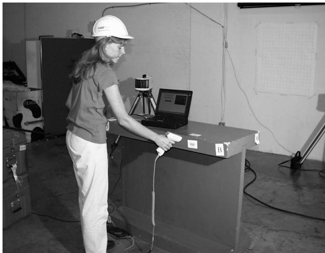
Figure 3b: Field Inspector acquires the component ID using a barcode scanner; the same information may be automatically acquired using non-contacting RFID technology. Part ID and coordinate acquisition tasks are integrated through a local laptop computer which is wirelessly connected to the Internet. Work is underway at NIST to integrate these functions into a compact, field portable device.
