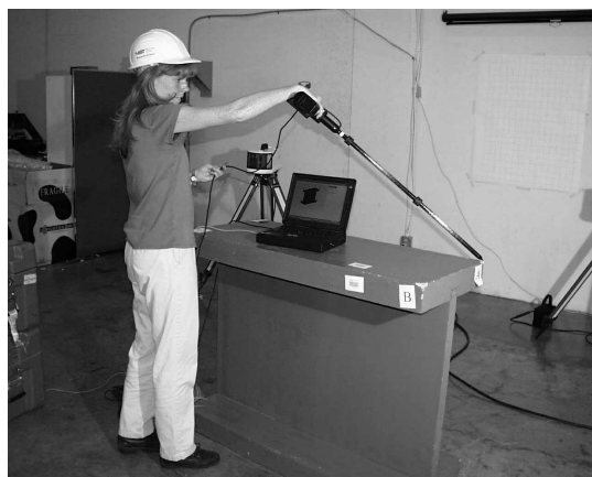
Figure 3f: The Field Inspector acquires at least three fiducial point locations (a process that takes about 30 seconds total). The part ID and the fiducial point coordinates are then wirelessly uplinked to the part localizer.
