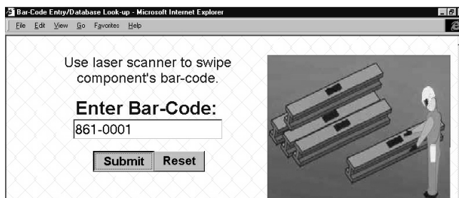
Figure 3c: A successful part identification brings up the component ID number. The Field Inspector then wirelessly submits a part query through the web for further information.
