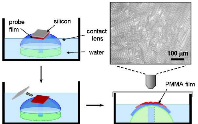
**Figure 1.** Schematic of experimental geometry for wrinkling of a sensor film (poly(methyl methacrylate) (PMMA)) on a contact lens. Optical microscopy is used to ascertain the wrinkling wavelength.
