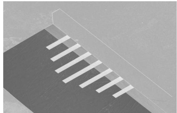
FIG. 3. Scanning electron micrograph of the experimental reference cantilever array. The cantilevers are nominally  $1.4 \mu\text{m}$  thick and  $50 \mu\text{m}$  wide and vary in length from 300 to 600  $\mu\text{m}$ .
