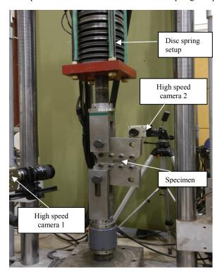
Figure 1: The dynamic apparatus.
