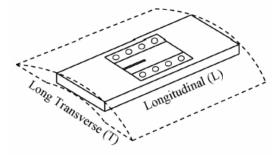
Figure 5: Orientation of CTOA specimen in the pipe.
