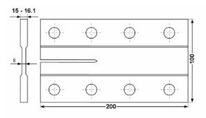
Figure 6: MDCB specimen, configuration and dimensions (mm).
