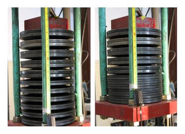
A. B. Figure 3: The spring setup (A) in the unloaded position and (B) in the maximum loaded position.
