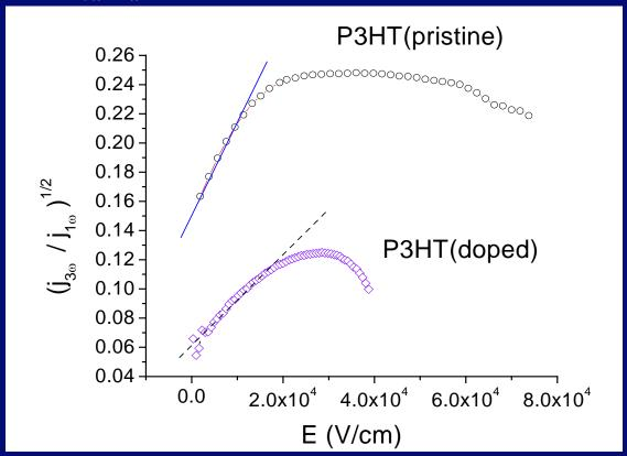
The non-linear charge transport is dominated by the third-order conductivity, which originates from extended  $\pi$ -type electronic states in P3HT
