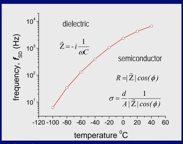
There is a definite frequency at a fixed temperature at which semiconducting to dielectric transition first occurs and we denote this frequency f<sub>SD</sub>.
