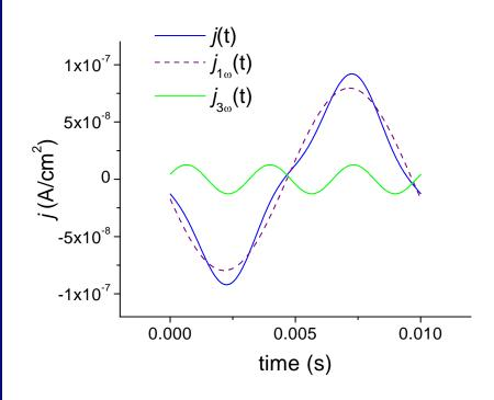
Calculating phasor transform of harmonics  $|j_{n\omega}|$  (n=1,3,...) by DFT
