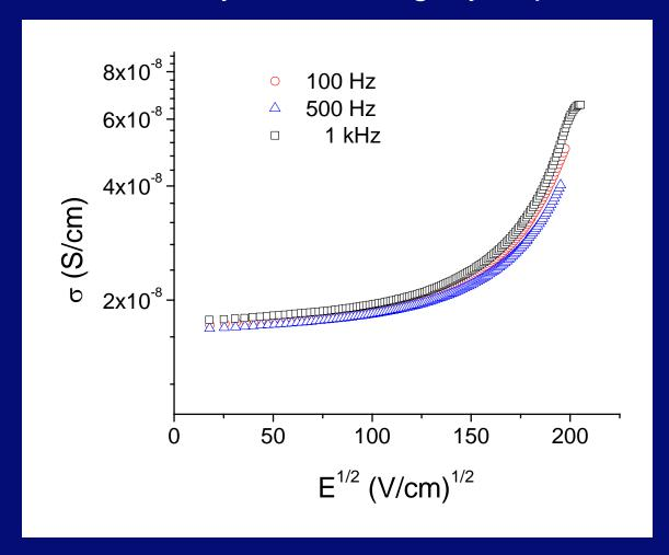
Lightly doped P3HT shows larger conductivity then P3HT(pristine) Field effect is insignificant at  $E < 1.5 \times 10^4 \text{ V/cm}$  Conduction mechanism appears similar to that in lightly doped PPy
