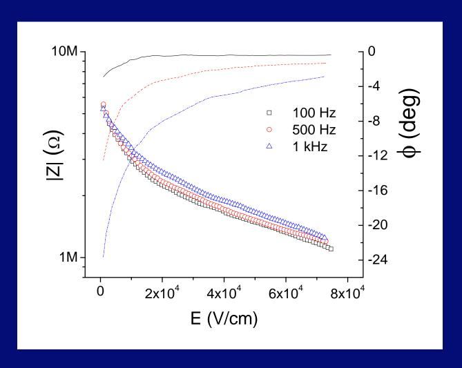
The impedance decreases with increasing electric field strength due to field activated charge transport
