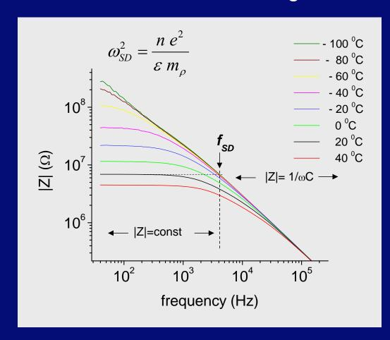
$f < f_{SD} |Z| = \text{const} = R \text{ semiconductor}, \ \phi = 0$   $f > f_{SD} |Z| = 1/\omega C \text{ dielectric}, \ \phi = -90^{\circ}$  $f_{SD} \text{ depends on temperature}$
