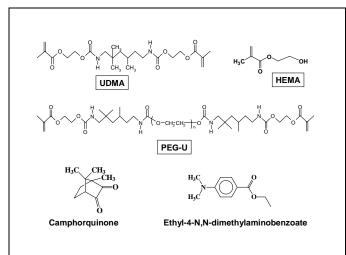
Fig. 1. Chemical structure of monomers and photo-initiator system.
