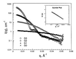
**Figure 2.** SANS curves for all generations at 30 °C. Inset shows a typical Guinier plot used to obtain  $R_{\rm g}$ .
