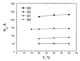
**Figure 3.**  $R_{\rm g}$  for arborescent graft polymers in *d*-cyclohexane versus temperature.
