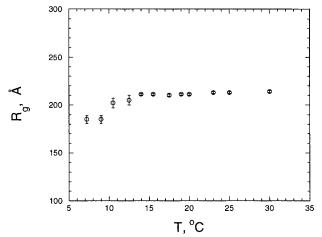
**Figure 10.**  $R_{\rm g}$  for generation 3 polymer in *d*-cyclohexane versus temperature showing the collapse of the molecule upon phase separation.
