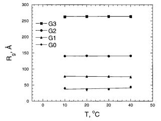
**Figure 4.**  $R_g$  for arborescent graft polymers in *d*-toluene versus temperature.
