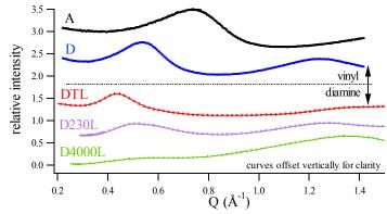
**Figure 2**. Wide angle X-ray scattering curves for several of the networks presented in Figure 1. The curves are normalized to the intensity of the strongest peak and then offset vertically in order of decreasing tether length, with the longest tether (D4000L) at the bottom and the shortest (A) at the top. The statistical uncertainty in the intensities is better than 5%.
