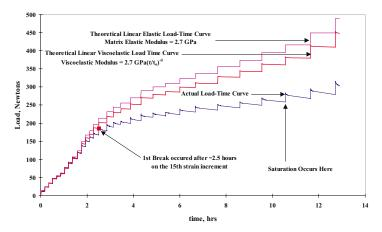
FIG. 1 Actual load-time curve with linear elastic and linear viscoelastic approximations for bare E-glass fiber SFF test specimen.
