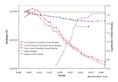
Figure 4. Variation of moduli with strain and number of fiber breaks.
