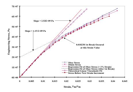
FIG 2. Pseudo-isochronal stress-strain plots for SFF test specimen containing a bare *E*-glass fiber (variable loading time increments).
