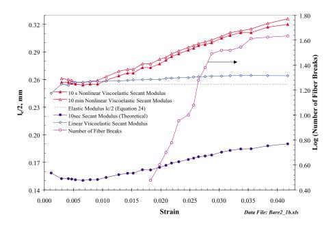
FIG 5. Variation of critical transfer length with strain and number of fiber breaks
