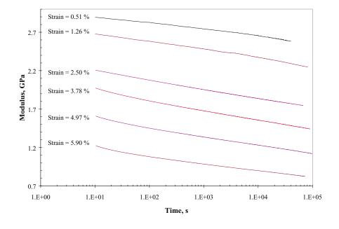
FIG 3. Single-step relaxation behavior of DGEBA/m-PDA dogbone specimens.
