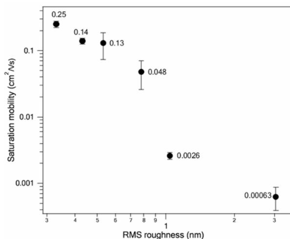
Figure 5. Charge carrier mobility ( $\mu$ ) plot for pBTTT thin film transistors after heating at mesophase for substrates of various dielectric roughness. Uncertainty in mobility measurements is the standard deviation calculated from the distribution of saturation field effect mobilities.
