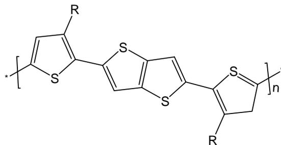
Figure 1. Chemical structure of poly(2,5-bis(3-alkylthiophen-2-yl)thieno[3,2-b]thiophene) (pBTTT).
