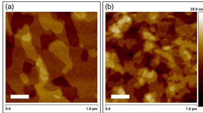
Figure 2. AFM images comparing microstructure of pBTTT on OTS (a) and oxide (b). Scale bar denotes 200 nm.
