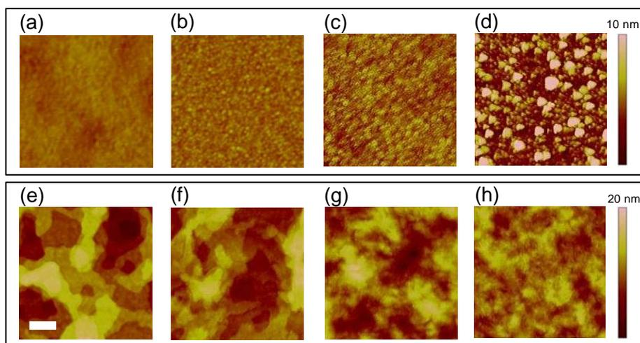
Figure 3. (a) – (d) AFM micrographs of rough oxides after OTS passivation. All images have 10 nm vertical scales. RMS roughness of (a) = 0.33; b) 0.53; c) 0.78; d) 3.04 nm. (e) – (h) AFM of pBTTT atop each rough surface after heating above mesophase transition and then cooling. All images have 20 nm height scales and are  $1 \mu\text{m} \times 1 \mu\text{m}$  size. Scale bar denotes 200 nm (4).
