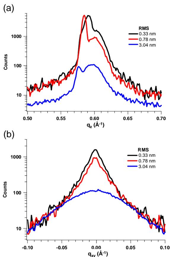
Figure 4. X-ray diffraction of annealed pBTTT on various roughness OTS treated substrates. (a)  $q_z$  and (b)  $q_{xy}$  of the (200) diffraction obtained from two-dimensional diffraction images near the Bragg condition (4).
