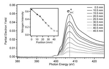
**Figure 3.** NEXAFS spectroscopy analysis for the statistical-copolymerbrush, PBMA-*co*-PDMAEMA, composition gradient. The inset shows the linear variation of nitrogen density with position.
