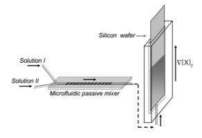
**Scheme 1.** Experimental setup for the formation of solution gradients inside a microchannel. Black arrows indicate the flow direction.  $\nabla[X]_{t}$ : change in concentration of solution X, with position, t.
