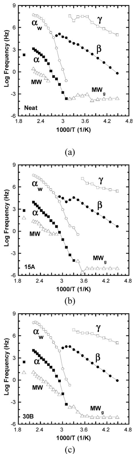
Fig. 10. Characteristic frequency in a logarithmic scale is plotted against reciprocal temperature for (a) neat nylon 6 (b) 15A-filled and (c) 30B-filled composite. The process  $MW_g$  refers to the Maxwell–Wagner relaxation that occurs below  $T_g$ .
