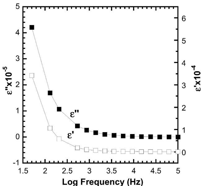
Fig. 5.  $\epsilon'$  and  $\epsilon''$  versus log frequency for nylon 6 with 4% 30B clay and processed at 242 °C.
