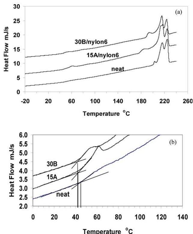
Fig. 1. (a) The DSC scans of neat nylon 6 and its composites with 15A and 30B clays. (b) DSC scans in the region of the glass transition. Vertical lines mark the glass transition temperatures.
