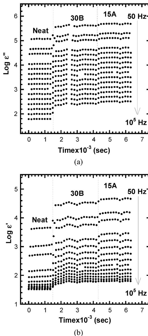
Fig. 4. Dielectric loss (a) and relative permittivity (b) were plotted versus time for compounding of nylon 6 with 30B and 15A clays. Data were obtained at the processing temperature, 242 °C.
