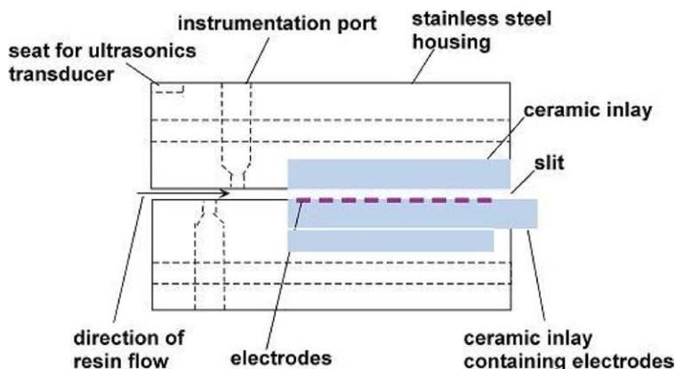
Fig. 3. Side view of the dielectric slit die.
