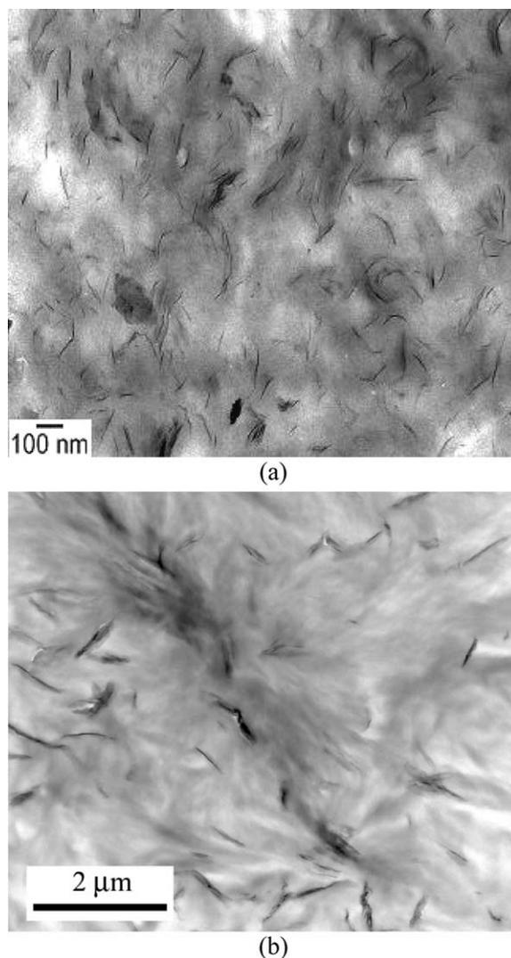
Fig. 2. TEM pictures of partially exfoliated 30B (a) and aggregated 15A (b) filled nylon 6 composites.
