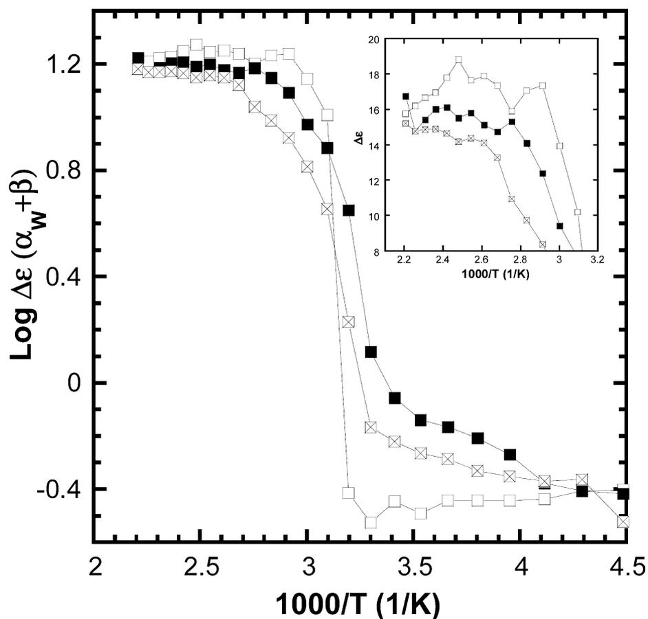
Fig. 17. Total dielectric relaxation strength summed from both  $\alpha_w$  and  $\beta$  relaxation was plotted versus reciprocal temperature for the neat nylon 6 ( $\square$ ), 15A-filled ( $\blacksquare$ ) and 30B-filled composite ( $\otimes$ ).
