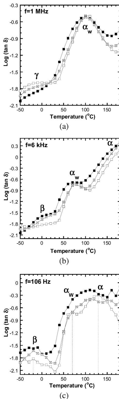
Fig. 6. Dielectric loss factor versus temperature at three experimental frequencies (a) 1 MHz (b) 6000 Hz (c) 106 Hz were plotted for the neat nylon 6 ( $\square$ ), 15A ( $\blacksquare$ ) and 30B ( $\boxtimes$ ) composites. In plot (c), in order to identify the  $\alpha$  relaxation in the high temperature regime,  $\sigma_{\text{DC}}$  estimated from the fitting was extracted from the raw  $\epsilon''$ .
