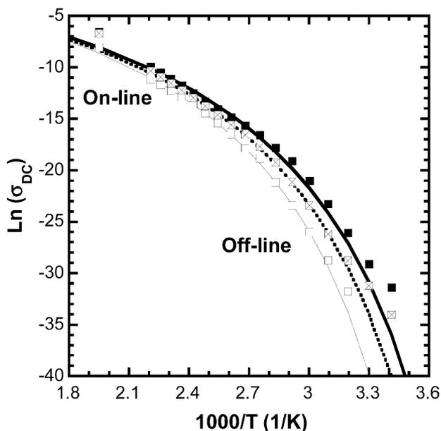
Fig. 11. DC conductivity ( $\sigma_{dc}$ ) is plotted against reciprocal temperature for the neat nylon 6 ( $\square$ ), 15A-filled ( $\blacksquare$ ) and 30B-filled composite ( $\boxtimes$ ). The lines through the data are the result of fitting the VTF equation to each data set. VTF fitting parameters are listed in Table 2. The average curve fitting error to these data ranges from 0.85 to 1.2%.
