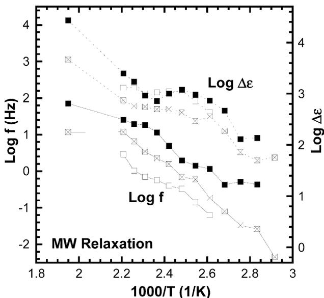
Fig. 13. Characteristic frequency and dielectric relaxation strength from Maxwell–Wagner interfacial polarization were plotted versus reciprocal temperature for the neat nylon 6 ( $\square$ ), 15A-filled ( $\blacksquare$ ) and 30B-filled composite ( $\boxtimes$ ).
