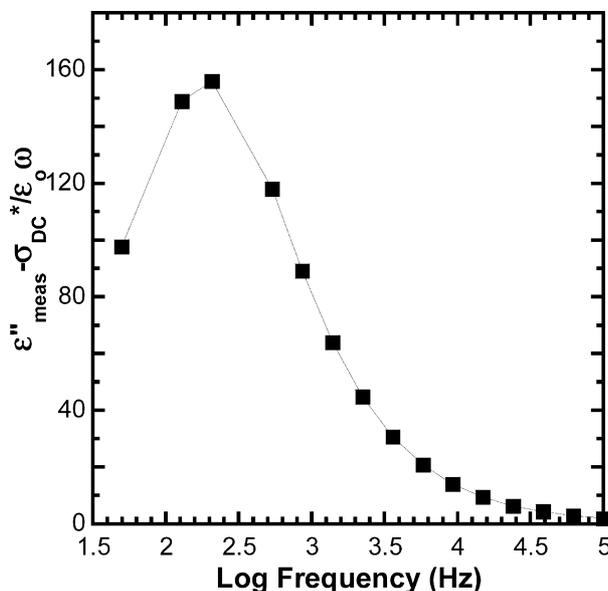
Fig. 8. Measured dielectric loss minus an estimated DC conductivity is plotted versus frequency for nylon 6 at 242 °C. The characteristic frequency at approximately  $\log f = 2.5$  is the value used to as an initial value to carry out the non-linear regression analysis.
