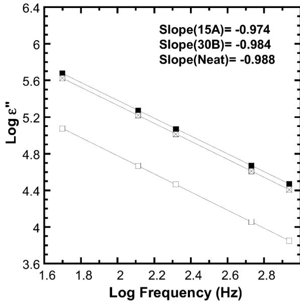
Fig. 7. Dielectric loss is plotted versus frequency on a log–log scale for nylon 6 ( $\square$ ), 15A ( $\blacksquare$ ) and 30B ( $\boxtimes$ ) composites at 242 °C. We note that the slopes for all three materials is greater than  $-1$ .
