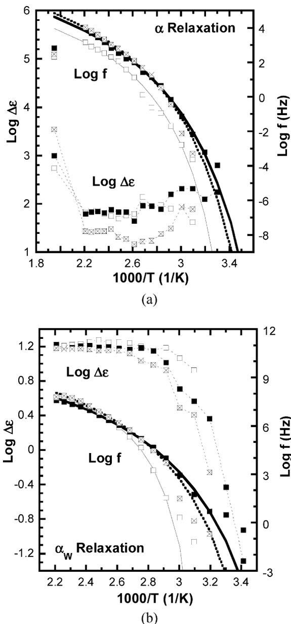
Fig. 15. Characteristic frequency and dielectric relaxation strength from (a)  $\alpha$  relaxation and (b)  $\alpha_w$  relaxation were plotted versus reciprocal temperature for the neat nylon 6 ( $\square$ ), 15A-filled ( $\blacksquare$ ) and 30B-filled composite ( $\boxtimes$ ). Lines through the data are the result of VTF fitting for which average curve fitting errors ranged from 0.91 to 5.4%.
