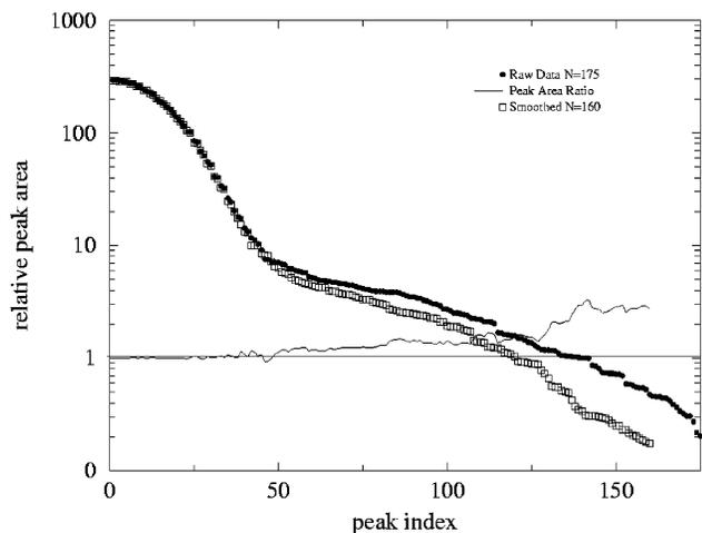
Figure 7. Relative peak areas sorted by size for the data of Figure 3 before (solid circles) and after (open squares) application of a 7-point moving average. Solid line is the ratio of relative peak areas before and after smoothing showing how ion intensity has been effectively smoothed away.
