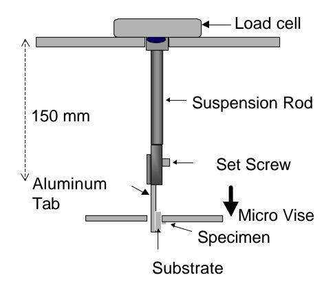
Figure 1: Schematic of the microshear test.
