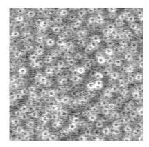
Figure 3. "Phase imaging" picture of a clay filled PMMA film (5  $\mu$ m x 5  $\mu$ m). TEM images of the clay particles show that they have an average size of about 100 nm.
