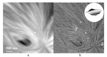
**Figure 1.** AFM image of the spherulitic morphology of an isothermal crystallized Polyamide 6 at  $T_c = 152^{\circ}C$ . a) "Height" image, b) "Phase" image. F = 263.8 KHz,  $A_0 = 18.6$  nm and  $r_{sp} = 0.7$ . Inset of figure 1b shows an individual lamella. Fine details are visible by Phase Imaging<sup>TM</sup>.
