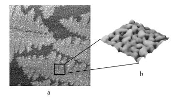
**Figure 2.** "Height" AFM image of the dendritic morphology for a clay filled PEO/PMMA blend. a) 20  $\mu$ m x 20  $\mu$ m, b) 3  $\mu$ m x 3  $\mu$ m. Phase separation is occuring within the PEO-rich dendrite.
