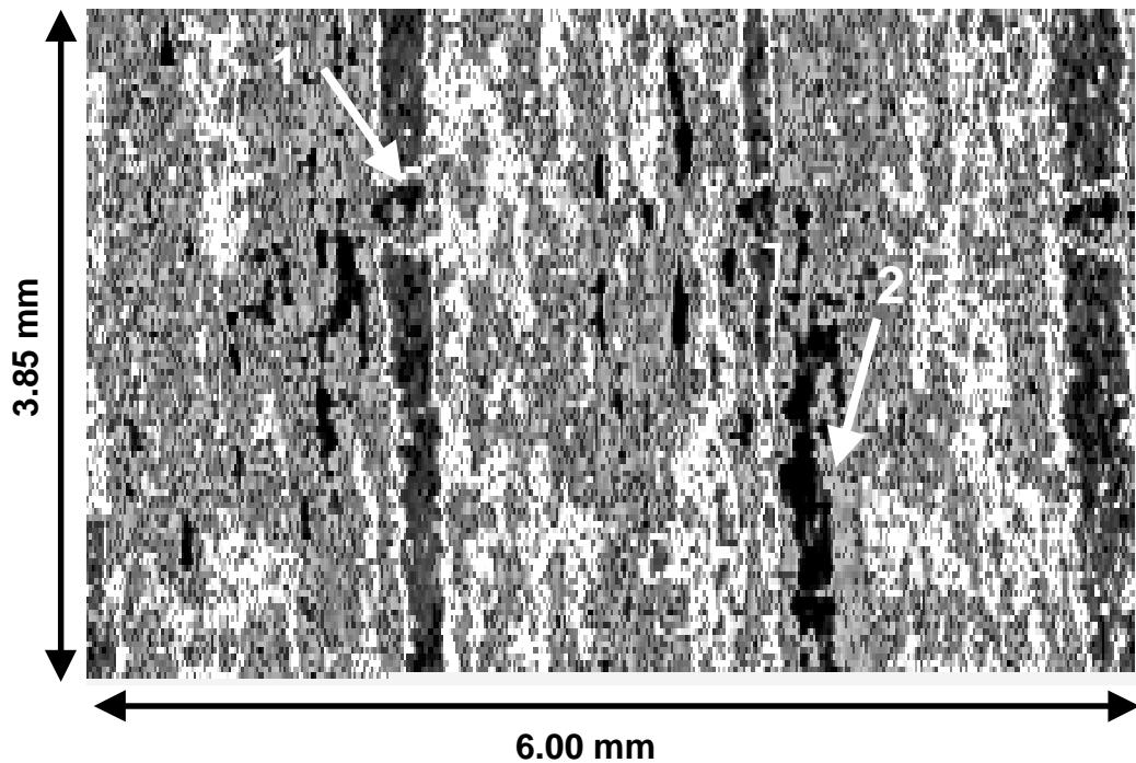
**Figure 2:** Cross-section of epoxy/unidirectional E-glass composite along the x-y plane at a depth of 740  $\mu\text{m}$ . Arrow 1 shows the stitching that holds the individual layers together. Arrow 2 indicates an elongated void within the tow.
