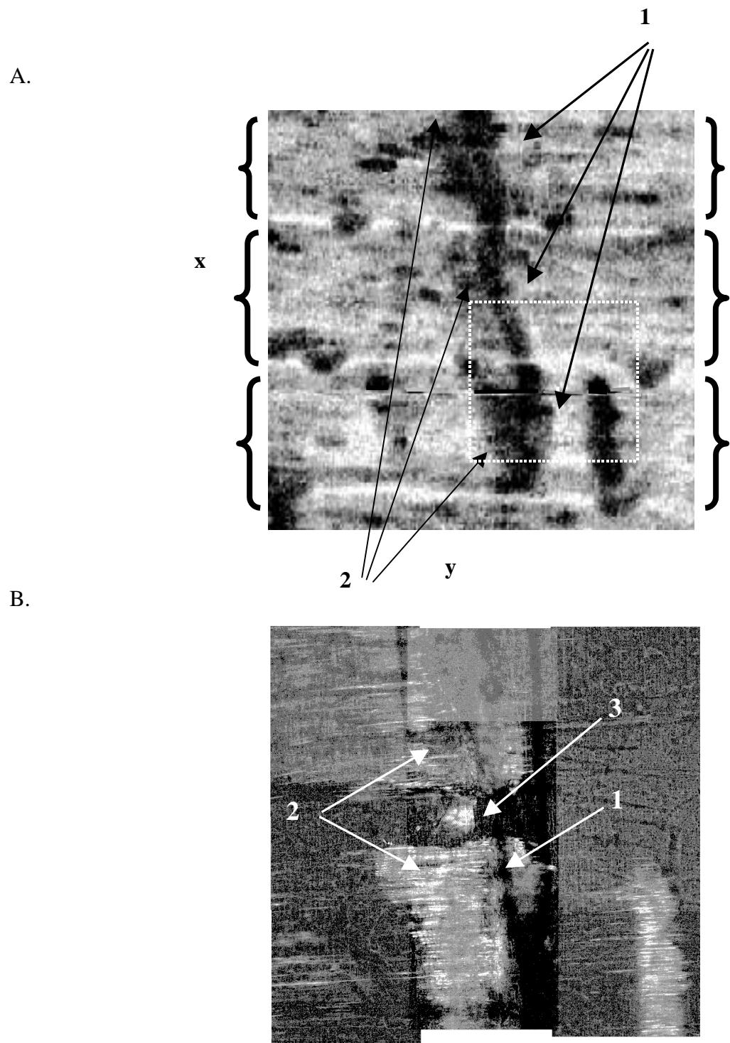
**Figure 3:** OCT (A.) and LSCM (B.) images 340  $\mu\text{m}$  from top surface of composite.
