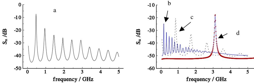
Fig.3. Measurement example using the microstrip test specimen. a) HADCO BC2000, the resonator length  $l=164$  mm,  $\epsilon^1 = 3.93$  at 461 MHz, b) HADCO EmCap,  $l=164$  mm,  $\epsilon^1 = 36.3$  at 151 MHz, c) HADCO EmCap,  $l=29.5$  mm,  $\epsilon^1 = 36.4$  at 842 MHz, d) HADCO EmCap  $l=8$  mm,  $\epsilon^1 = 35.9$  at 3.122 GHz
