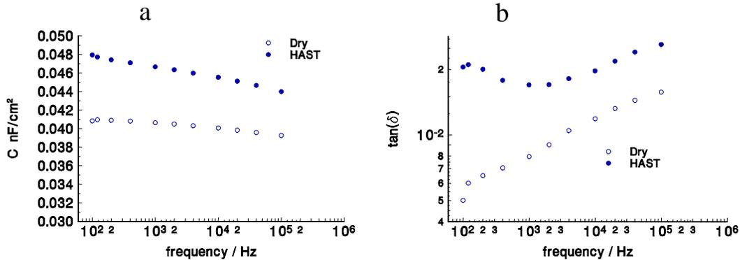
Fig.6. Capacitance density (a) and the dielectric loss tangent (b) of FR4 saturated with moisture during HAST. (TV0 / Merix, pattern C)
