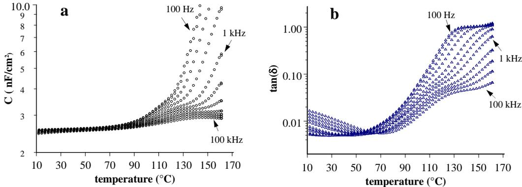
Fig.10. Capacitance density (a) and the dielectric loss tangent (b) of C-Ply as a function of temperature and frequency.(TV0 /3M, pattern B)
