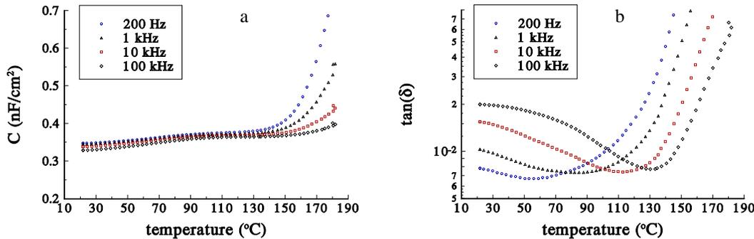
Fig.8. Capacitance density (a) and the dielectric loss tangent (b) of EmCap as a function of temperature and frequency.(TV0 / MERIX, pattern B)
