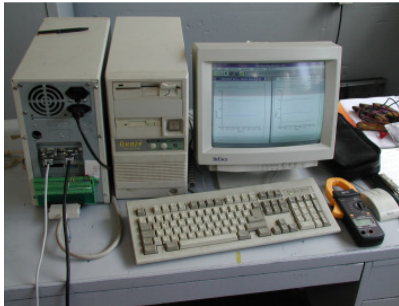
Figure 2. Photo of the on-line arc-welding monitor.
