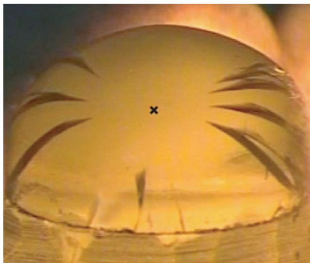
**Fig. 11.** Front-on view of off-axis contact fracture of epoxy-filled glass domes,  $d = 1$  mm and  $r_s = 6$  mm, on epoxy base. Indentation with teflon disk at 1000 N. Note how margin cracks initiate and propagate around side of dome toward contact center (cross) to form "tiger" pattern. Courtesy Mahek M Shah and Vibhu P Saxena.
