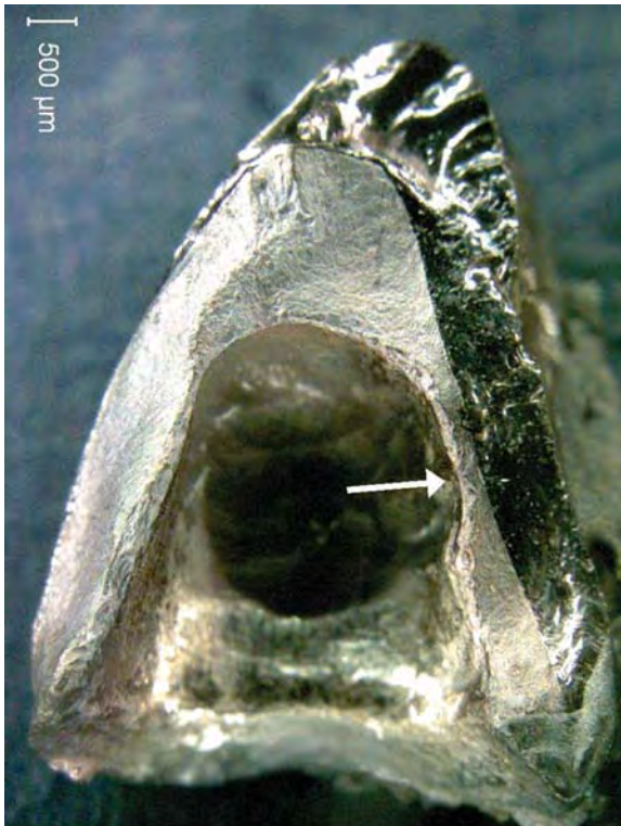
Figure 10.30 f-g. (f) shows an SEM image wake hackle in the glassy veneer from a region near the top (occlusal) surface of the A half. The wake hackle shows that the crack was running in the direction of the arrow in this region. All the wake hackle in the entire crown showed fracture was from the inside to the outside. (g) shows the origin site is a cone crack on the inside surface (arrow). The following photos show this site in more detail.
