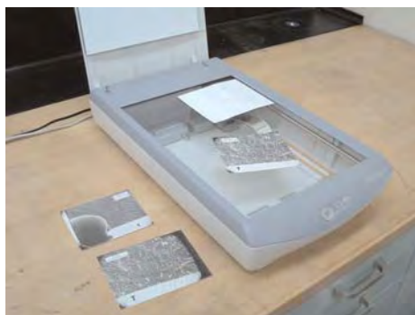
Figure 3.53. Other useful equipment for a fractography laboratory. Digital scanner (a) and ultrasonic cleaning bath (b).
