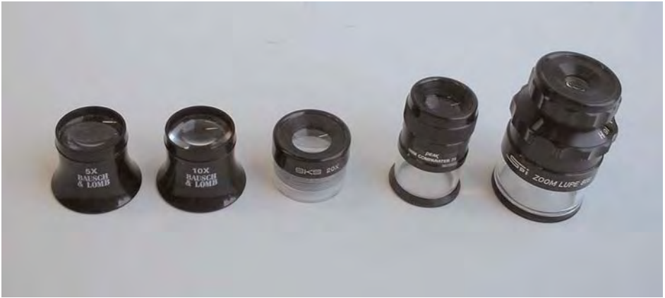
Figure 3.2. Hand loupes and optical comparators. From the left, 5 X and 7 X watchmaker loupes; a 20 X loupe, a 7 X comparator with an internal 20 mm scale marked in 0.1 mm increments, and a 8 X to 16 X zoom comparator with an 16 mm scale marked in 0.1 mm increments.
