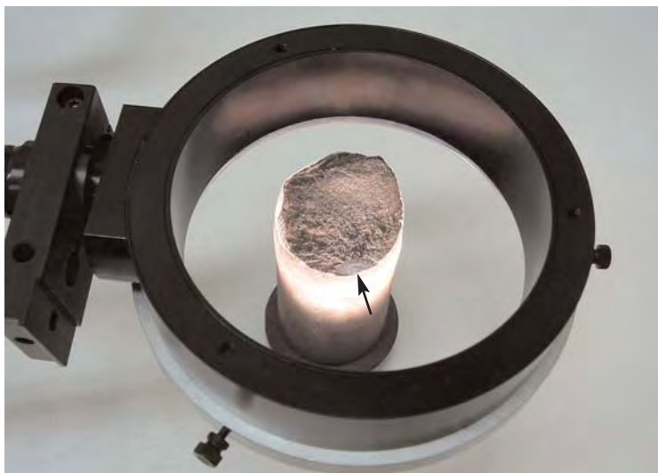
Figure 3.16. Dark field illumination of the fracture surface of a fractured steel railroad coupler pin. The arrow points to a fatigue crack.
