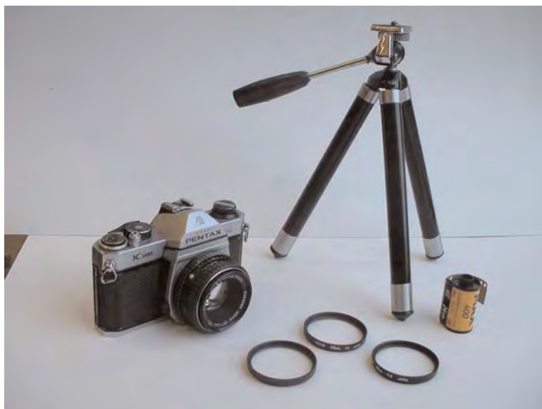
Figure 3.8. 35 mm single lens reflex camera with conventional film, tripod, and close-up lenses.
