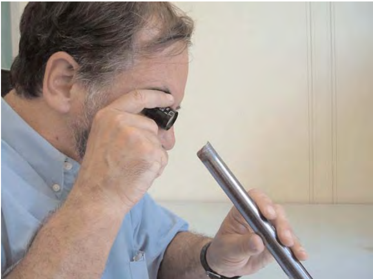
Figure 3.3. Loupes (5 X to 20 X) may either be held by the eye or by hand. The part is a single crystal silicon rod.
