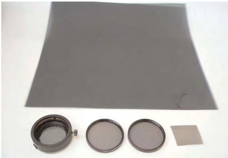
Figure 3.19. Crossed polarizing filters or plastic sheets. Polarizers can either be dedicated accessories for the stereoscope, or can be improvised from ordinary single lens camera lens attachments or sheets of plastic polarizing film.
