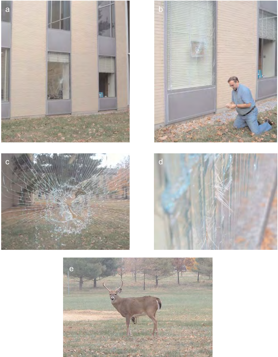
Figure 4.15 Window fracture problem. Evidence collected at the scene included foreign material attached to the impact site as shown in (d). The crack patterns indicated impact from the exterior. That plus the height of the impact above the ground, the tuft of fur, the time of the year (November, the rutting season) and similar occurrences elsewhere suggested the cause of failure shown in (e).
