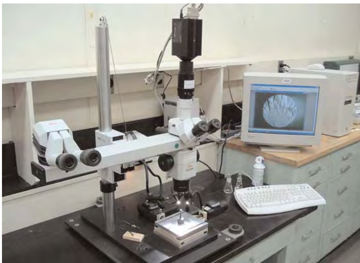
Figure 3.12. A discussion stereoptical microscope that allows two observers to simultaneously view an object. Note the very tall post (800 mm) on which the microscope body is mounted. The entire assembly can be moved up or down as required to facilitate examination of very large or very small specimens. Beam splitters in the optical path enable simultaneous viewing through the eyepieces at the same time the digital camera views the object. The digital camera is connected to a computer and monitor.
