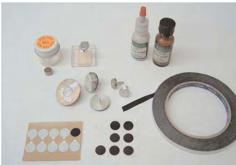
Figure 3.35. SEM specimen preparation tools. Clockwise from the top left are two SEM length calibration standards, two silver paint bottles, a double-sided conductive adhesive tape roll, two sheets of double-sided conductive adhesive disks, and an assortment of aluminum stubs.
