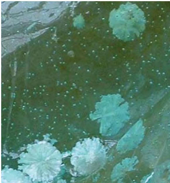
Figure 6.31. Unusually large ( \approx 1 cm) glass devitrification inclusions with a blossom like structure as well as smaller seed bubbles. (Specimen courtesy of J. Varner and V. Fréchette)
