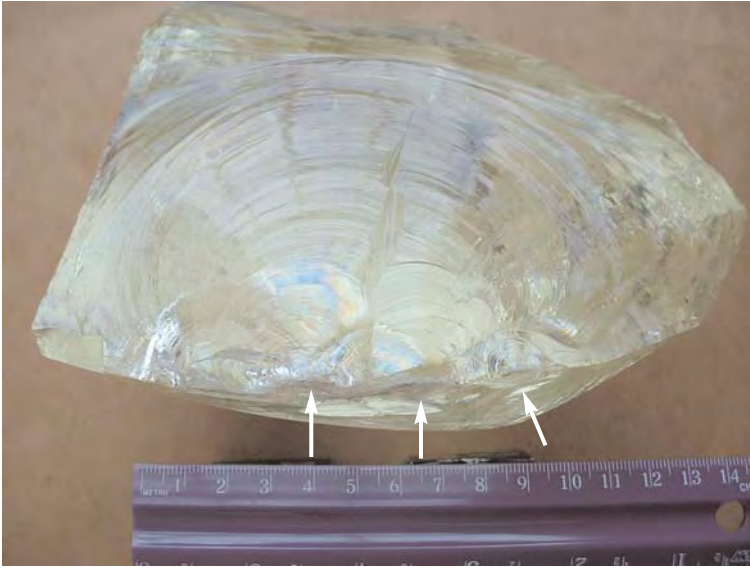
Figure 5.34 Tertiary Wallner lines in a large chunk of glass that was hammered into pieces. There are multiple impact sites marked by arrows, the most prominent of which is marked by the larger white arrow. Notice how the tertiary Wallner lines are concentric about the impact sites. This was one of Professor Fréchette's demonstration pieces.
