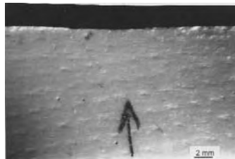
Figure 10.22. Sintered fused silica radome that fractured during a proof test. (a) is a top view with the origin region marked by the arrow. The ceramic is bonded on the inside to a fiber epoxy attachment ring. (b) is a schematic showing the attachment scheme. Fractures in the ceramic typically occurred near the top of the thread ring. (c) shows a grinding crack at the origin area (arrows). (d) shows a grinding pattern on the inside ceramic surface.
