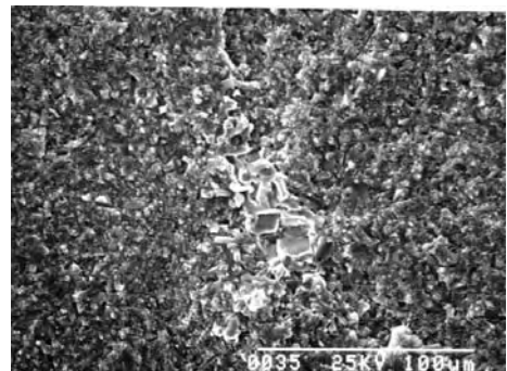
Figure 6.48. Multiple photos should be taken showing whole fracture surface, the mirror region and the origin. The right side shows an example for an inclusion in a silicon nitride rod flexural strength specimen.
