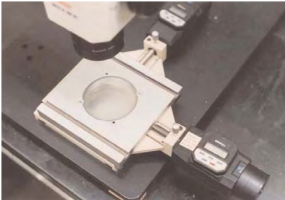
Figure 3.24. A X-Y traversing stage with digital micrometer heads is very convenient for positioning a specimen and also for making accurate size readings.
