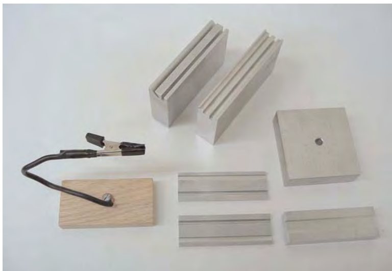
Figure 3.5. Specimen holders. Clockwise from the lower left are: a bend bar holder made with an alligator clip on a bendable (10 gage electrical) wire with electrical tape wrapped around the teeth to cushion the specimen, two aluminum jigs with slots and grooves for bend bars or tension strength specimens, an aluminum block with hole, and three aluminum holders comparable in size to a glass microscope slide with grooves to hold bend bars both on their flats and on edge for chamfer examination.
