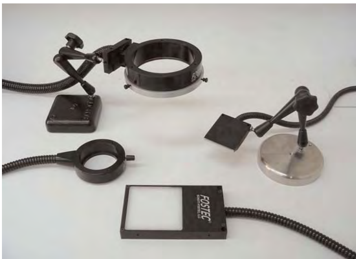
Figure 3.13. Illumination sources for use with a stereomicroscope. Clockwise from the middle left: a ring light intended to be clamped to the objective lens, a ring dark light illuminator on an adjustable stand, a line light source on a stand, and a transmitted light platform.
