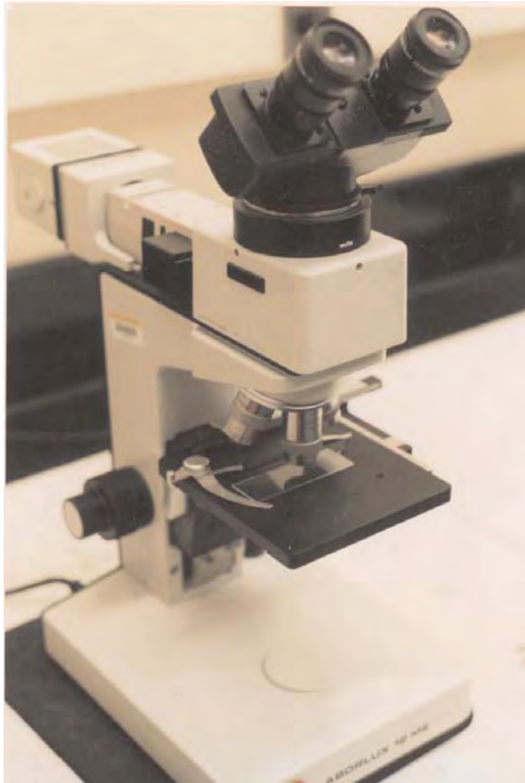
Figure 3.25. Compound reflected light microscope. Although the microscope has twin eyepieces, they both view the same image collected by the objective lens. Overall magnifications can be as much as 1000 X, but the working distances and the depths of field are very small. Only relatively flat specimens may be examined.
