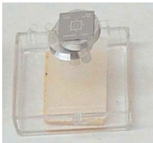
Figure 3.43. A NIST Standard Reference Material SEM length calibration standard. Finely spaced reference lines are located at intervals along the sides of the box on the right close up view.
