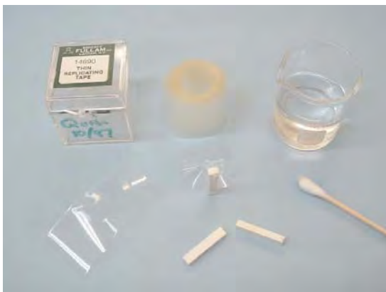
Figure 3.29. Thin cellulose acetate replica tape, acetone, applicator, and bend bar specimens.
