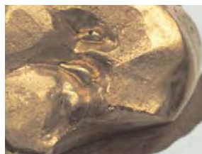
Figure 3.31. Steps in the preparation of a dental replica that is a positive duplicate of a fractured crown. Figure 6.50 has additional views of this fractured crown.
