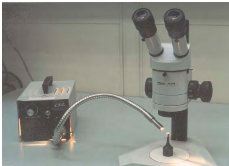
Figure 3.11. Stereo binocular microscope with a fiber optical light source for directional illumination. This is an indispensable tool for the ceramic and glass fractographer. Low incident angle or "vicinal illumination" is illustrated in the picture. In other cases, a ring light mounted on the objective lens of the microscope may be suitable. This particular microscope has interchangeable 0.63 X, 1.0 X and 2.0 X objective lenses, a body zoom magnification range of .65 X to 4 X, and 25 X eyepieces for an overall magnification range of 10 X to 200 X. The moderately tall (300 mm) mounting post enables large specimens up to 150 mm tall to be placed under the microscope.
