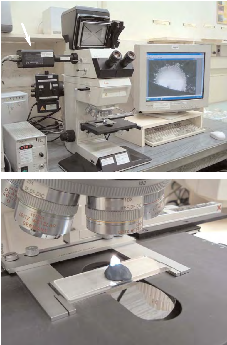
Figure 3.26. A research compound microscope with a digital camera and computer installation. Linear encoders with a 1 micrometer resolution are attached to the traversing X-Y stage and facilitate rapid size measurements. The instant film camera on the top was a common accessory in the 1970s to 1990s, but has been rendered obsolete by digital cameras such as the one marked by the arrow. A fractured glass rod mounted on blue polymeric clay is on the stage. The fracture mirror can be viewed through the eyepieces at the same time it is projected on the monitor.
