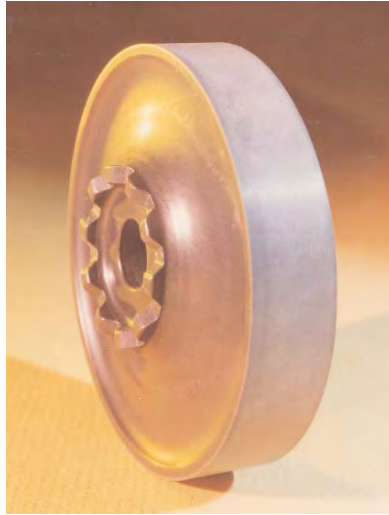
Figure 10.1. A Ford silicon nitride model gas turbine rotor which survived 25 h intact. The model rotor has a 95 mm diameter.
