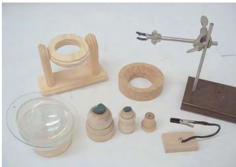
Figure 3.6. Component or specimen holders. Clockwise from the lower left: a homemade plastic platform mounted on a swivel base; a pivoting wooden holder; a cork ring; a clamp on a stand, an alligator clip on a stand, an inverted miniature wood flower pot with a hole, and two wooden candleholders with dolls heads and polymer mounting clay. The balls can be rotated to obtain optimum illumination angles onto the specimen's surface.
