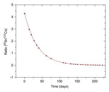
**Fig. 3.** HPGe measurements of the activity of the <sup>82</sup>Sr source No. 1952 in time. *R* is the ratio of the net gamma-ray emission rate of the 776.517 keV <sup>82</sup>Sr gamma-ray to the corresponding value of the 661.657 keV <sup>137</sup>Cs gamma-ray line.
