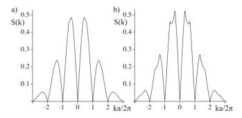
FIG. 5. Structure factor of the atomic mixture, with the same parameters as in Fig. 4, in  $1/\mu m$ , as a function of k in units of  $2\pi/a$ . (a) corresponds to very weak interactions  $U_{12}/U=0.0025$  and shows no particular structure beyond a SF signature; (b) corresponds to  $U_{12}/U=0.04$ . We see additional peaks, which indicate CDW QLRO at a momentum that is consistent with the density at the center of the trap.
