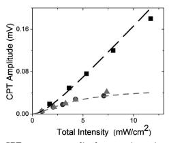
Fig. 4. CPT resonance amplitude versus intensity with optimal phase delay for the case of both fields (squares) and of a single field (circles, triangles).
