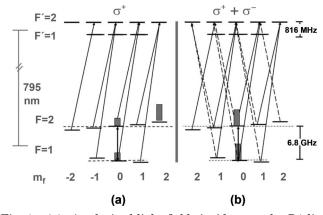
Fig. 1. (a)  $\sigma^+$  polarized light fields incident on the D1 line of <sup>87</sup>Rb in  $\Lambda$  configuration. A large fraction of atoms is lost to the  $|F=2, m_f=2\rangle$  state, resulting in a loss of CPT resonance signal. (b) A combination of  $\sigma^+$  and  $\sigma^-$  light fields can be used to accumulate a maximum number of atoms in the CPT dark state on  $m_f=0:0$  ground states.
