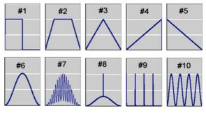
Figure 6. Ten different pulse waveforms used in the analysis.
