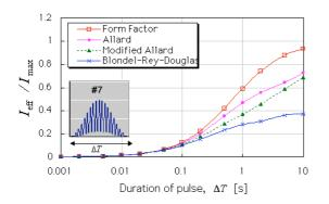
Figure 9. Results for a modulated pulse.
