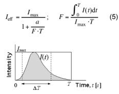
Figure 3. Schematic of the Form Factor method.
