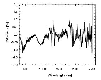
Fig. 7. Difference in sphere radiance measured by the GER Mark V IRIS instrument on the 18th of June. The measurements were made approximately 15 min apart.
