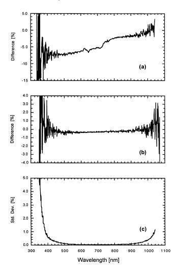
Fig. 4. Difference in sphere radiance measured by (a) the SDSU PSII and (b) the GSJ PSII 1 h apart. (c) The standard deviation of the mean of 10 scans averaged for one SDSU PSII sphere radiance measurement.
