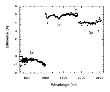
Fig. 8. Difference in sphere radiance measured by the GER 3700. Measurements were made approximately 1 h apart on the 18th of June. A Si array detector was used for region (a), a PbS array detector for region (b), and a second PbS array detector for region (c).
