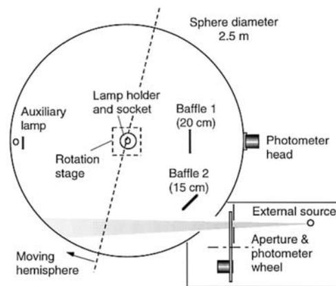
Figure 5. Arrangement of the new NIST 2.5 m integrating sphere (top view).
