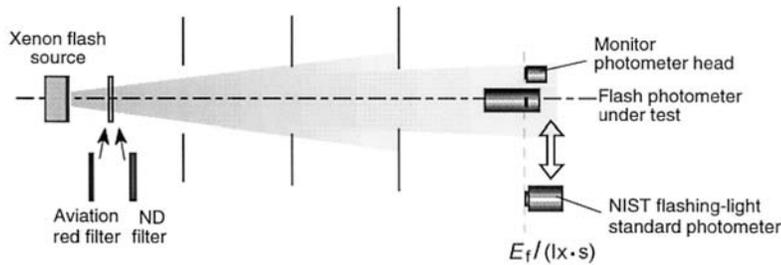
Figure 4. Arrangement for the calibration of flashing-light photometers.
