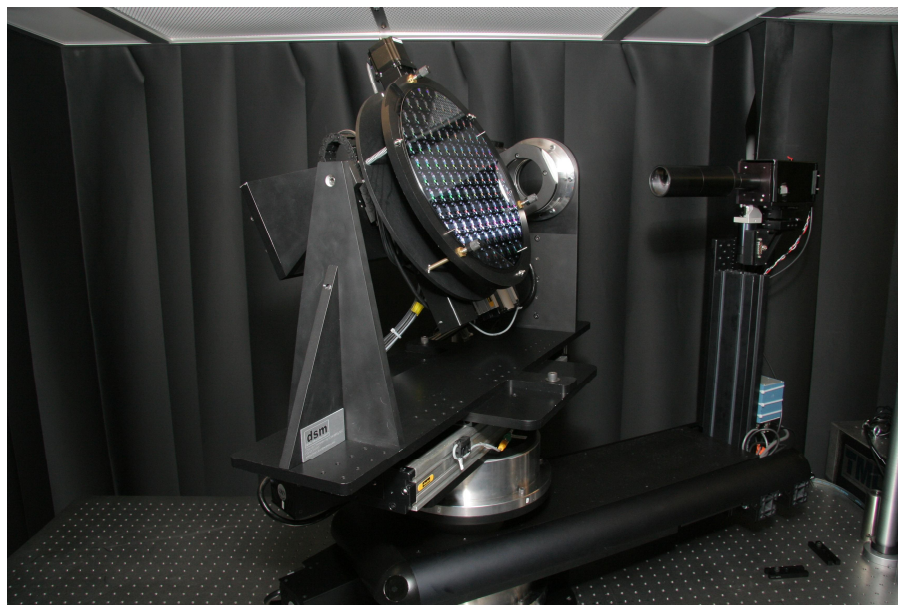
FIG. 1. The goniometric optical scatter instrument (GOSI), with 300 mm wafer on stage and scatterometry detector arm in place.
