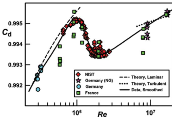
▲ International comparison of flow standards using four nozzles as a transfer standard conducted between 3,000 slm and  $3.6 \times 10^5$  slm. The discharge coefficient,  $C_d$ , equivalent to actual flow divided by model flow, is plotted as a function of the Reynolds number (Re). Laboratories are consistent because the four sets of data fall within 0.05 percent of a single curve. The jog in the curve near  $Re = 1.5 \times 10^6$  indicates the transition from laminar flow to turbulent flow.
