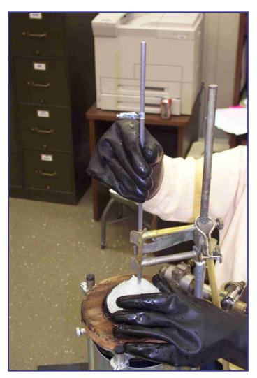
Use a clean rod (metal or glass) to make thermometer hole, prior to insertion of thermometer.
