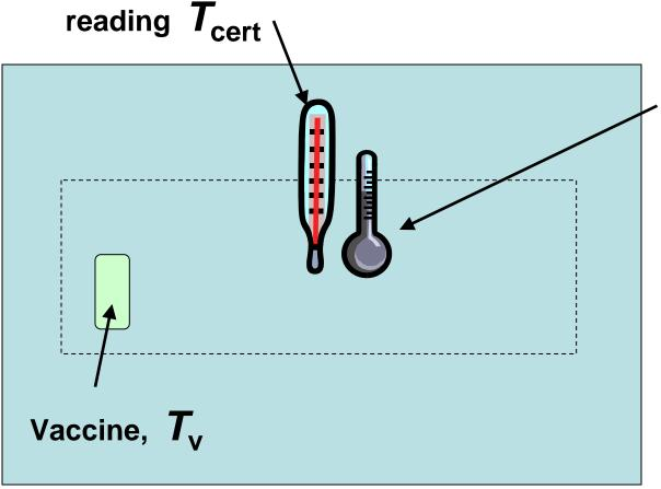
Redundant check thermometer, reading  $T_{\rm check}$
