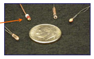
NTC: Negative Temperature Coefficient - The vast majority of commercial thermistors used as thermometers are in the NTC category.
