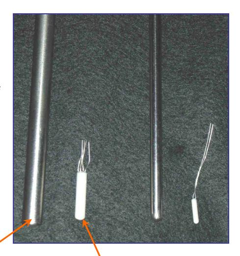
Steel sheath containing sensor Sensor or element (wire-wound shown)
