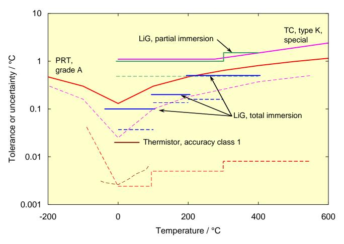
Colored lines: ASTM tolerances (ASTM E1, E1137, E230, and E879).
