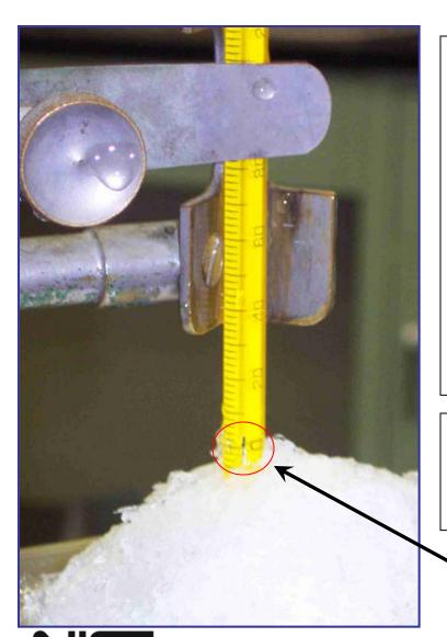
Thermometer in an Ice Melting Point
