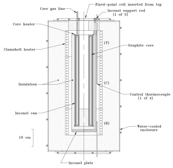
**FIGURE 1.** Schematic cross section of the four-zone furnace. The outer enclosure and heater wiring are not shown. (T), (C), and (B) indicate the top, center, and bottom zones, respectively.
