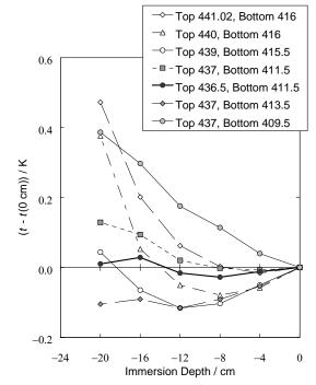
**FIGURE 2.** Immersion profiles in a silver freezing-point cell at a temperature 2 K above the freezing point, for a variety of furnace settings. For all profiles, the center zone was set at 417.5 (set point units approximately equal to  $10 \,\mu$ V).
