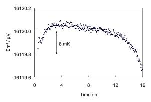
**FIGURE 4.** Freezing plateau of a silver freezing-point cell, as measured with a Au/Pt thermocouple.
