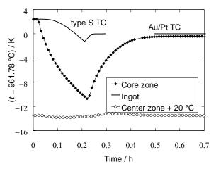
**FIGURE 3.** Temperature at full immersion in the well of the fixed-point cell ingot and of the center and core zones of the furnace during initiation of a freeze.
