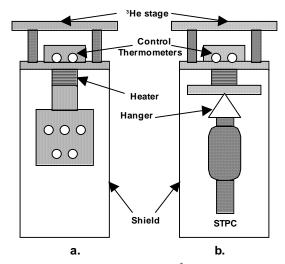
**FIGURE 3.** Controlled platform of  ${}^{3}$ He system shown in both operating modes: a.) with block installed as an isothermal comparator. b.) with STPC arranged as a calorimeter.
