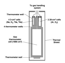
**FIGURE 1** Copper block containing cells for realization of the ITS-90 below 84 K.
