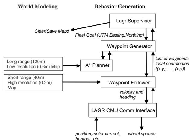
**Figure 10. Behavior Generation High Level Data Flow Diagram.**
