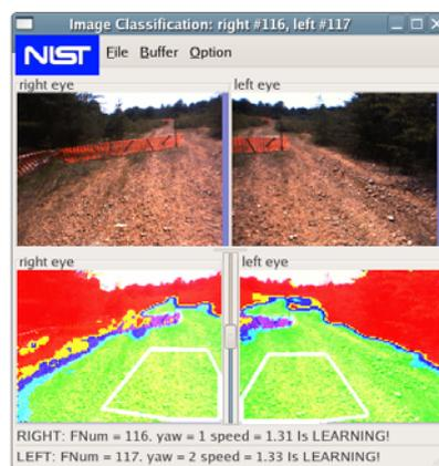
**Figure 7. OCU display showing original images (top) and cost images (bottom). The 1 m wide by 2 m long rectangular areas assumed to be ground (white boxes) are overlaid on the cost images.**
