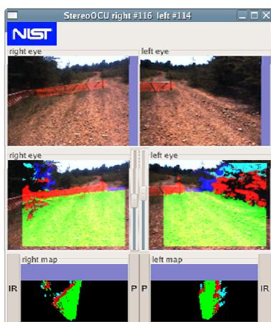
**Figure 6. OCU display showing original images (top), results of obstacle detection (middle), and cost maps (bottom). Red represents obstacles, green is ground, and blue represents obstacles too far away to classify.**
