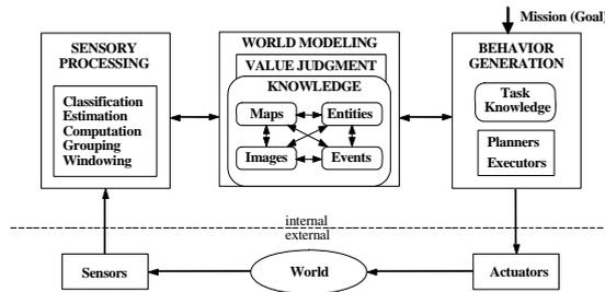
Figure 3. The basic internal structure of a 4D/RCS control loop.
