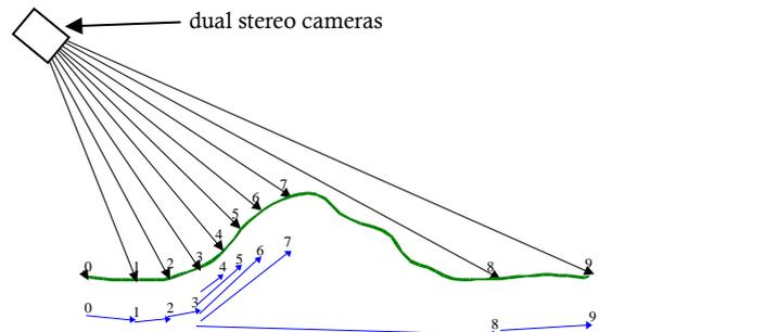
Figure 5. A single vertical scanline detecting the ground. Pixel 0 is altered to correspond to the bottom of the vehicle wheel. Pixels 1, 2, 3, 8 and 9 are ground pixels due to shallow slopes. Pixel 4, 5, 6 and 7 are obstacles due to steeper slopes. The slopes are shown by the direction vectors on the bottom of the figure.
