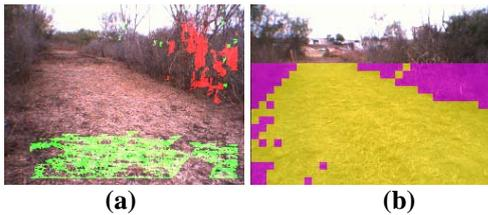
**Figure 11 Learning by example images.** (a) is an image taken during learning and overlaid with (red) obstacles and (green) ground, (b) is the same image overlaid with traversability information as obstacles (magenta) and ground (yellow).
