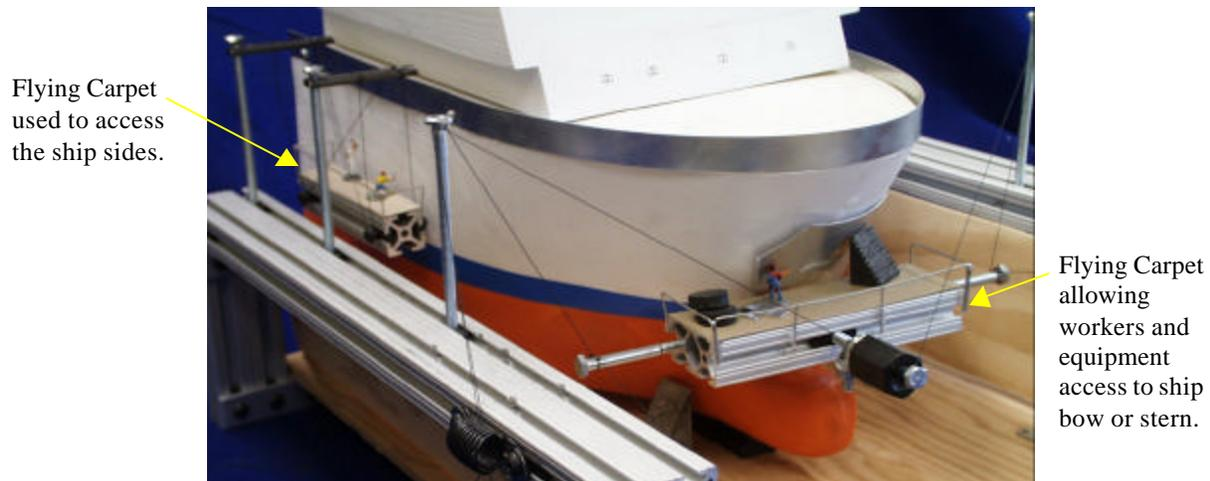
**Figure 10 –NIST Flying Carpet 1/120<sup>th</sup> scale model** applied to dry dock ship repair and conversion.
