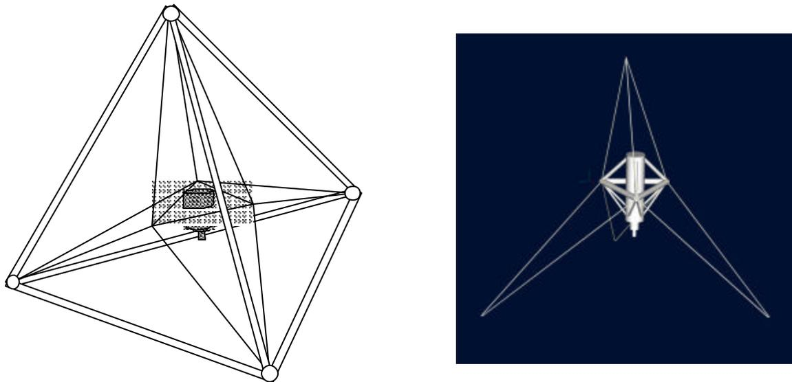
**Figure 5. Cable-Actuated Machine Tool** mounted in a tetrahedral tubular frame. (left) schematic drawing, (right) solid model rendering of a spindle platform and nine-cable mechanism without frame. (Winches not shown in either view.)
