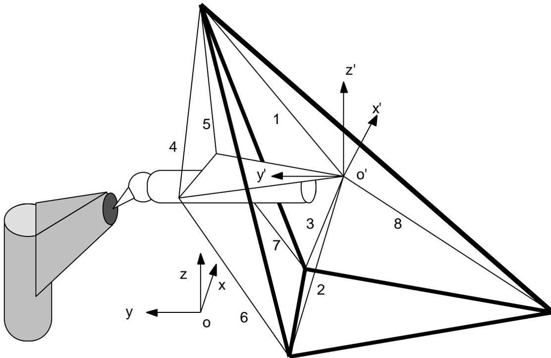
**Figure 9. A Macro Stereo-Lithography Machine.** On the right is the tetrahedral frame supporting the tool platform by 8 cables. On the left is a part of a structure that is being built up by depositing material from the extrusion nozzle.
