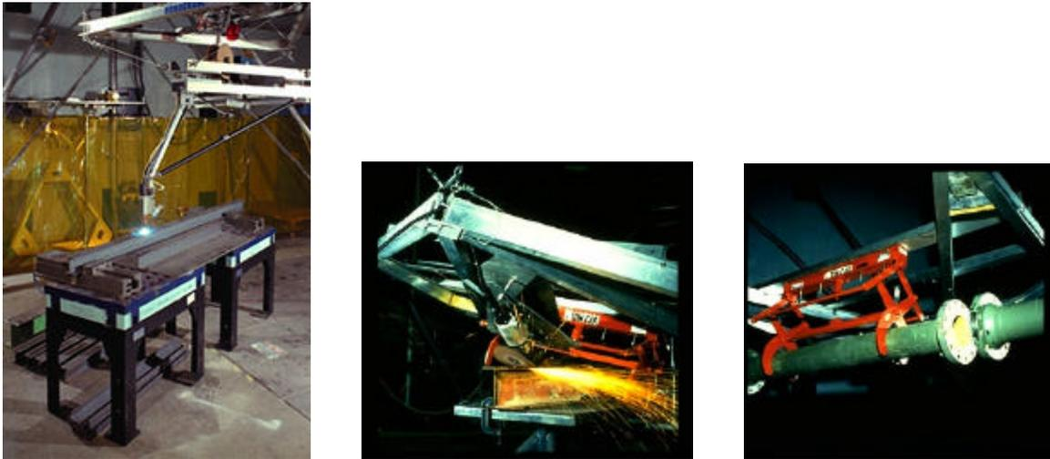
**Figure 3 –RoboCrane performing three different tasks.** (left) welding, (middle) grinding a weld bead, and (right) pipe-fitting flanged cast iron pipe.
