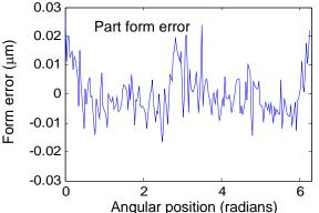
FIGURE 4 Part form error obtained as half the sum of the mean of 10 runs in Fig 2 and Fig. 3
