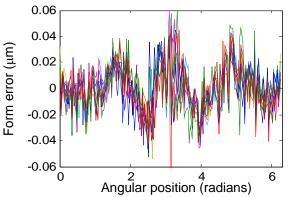
FIGURE 3 Radial form data from 3 mm sphere at the 180° position of a full Donaldson reversal, with 180 sampling points per trace and 10 traces
