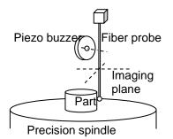
FIGURE 1. Schematic of the setup showing part mounted on a precision spindle, and the fiber excited acoustically. A piezo buzzer (which does not physically contact the fiber) generates the acoustic excitation.
