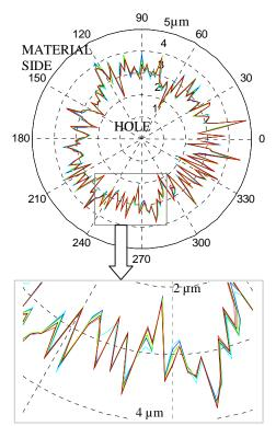
FIGURE 6 Radial form data from a knife-edge aperture. 180 sampling points per trace, 10 traces are shown. The repeatability at any location is only of the order of 62 nm. The out-of-roundness of this artifact is approximately  $2 \,\mu$ m.
