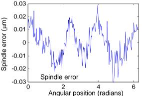
FIGURE 5 Spindle error obtained as half the difference of the mean of 10 runs in Fig 2 and Fig. 3
