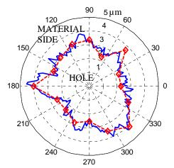
FIGURE 7 Radial form data from a knife-edge aperture used in NIST round robin comparison. 180 sampling points per trace, average of 10 traces shown in solid line. Additionally, the dashed-diamond line represents 16 sampling points measured with the probe on a CMM. 2D point coordinates were determined at each sampling location. The residuals from a Least Squares best fit circle are shown here.
