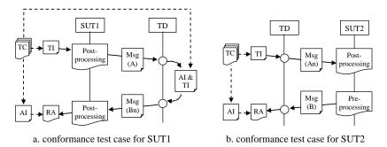
Fig. 6. Generated conformance test case for SUT2 (TC: test case, TD: test driver, Msg: message, Msg An: nominal message based on message A, and Msg Bn: nominal message based on message B)
