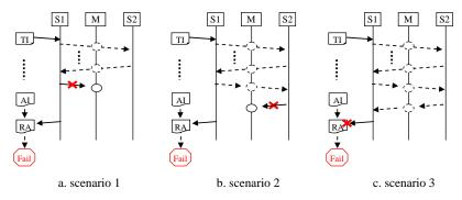
**Fig. 5.** Failed interoperability scenarios (TI: test instruction, AI: assert instruction, and RA: result analysis, S1: SUT1, S2: SUT2, and M: monitor)
