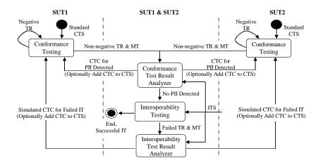
**Fig. 3.** Proposed iterative test procedure (CTS: conformance test suite, ITS: interoperability test suite, CTC: conformance test case, TR: test result, MT: message trace, IT: interoperability test, and PII: potential interoperability issue)
