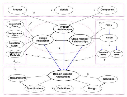
Figure 12: Modular product platform construction process, representation and reuse
