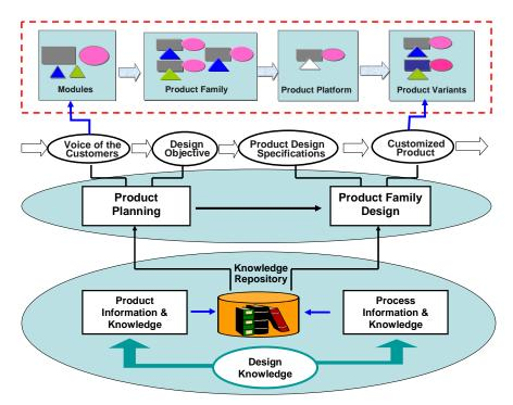
Figure 8: Knowledge support framework for module-based product family design
