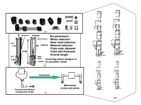
Figure 13: (a) Robot modules and library, (b) module attribute parameterization, (c) assembly / configuration, and (d) robot families
