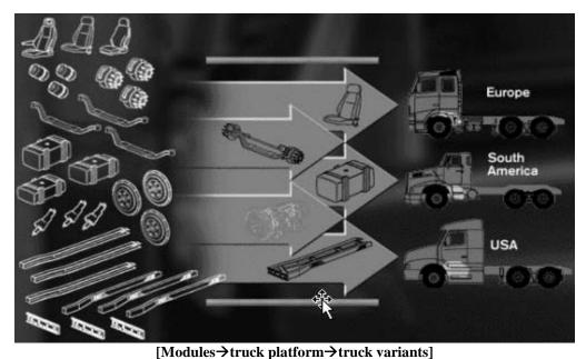
Figure 1: Modular truck family design and development (Courtesy of Volvo)
