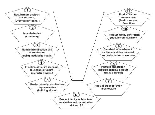
Figure 7: Module-based product family design for mass customization
