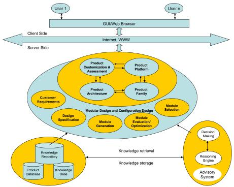
Figure 14: Web-enabled knowledge support system architecture
