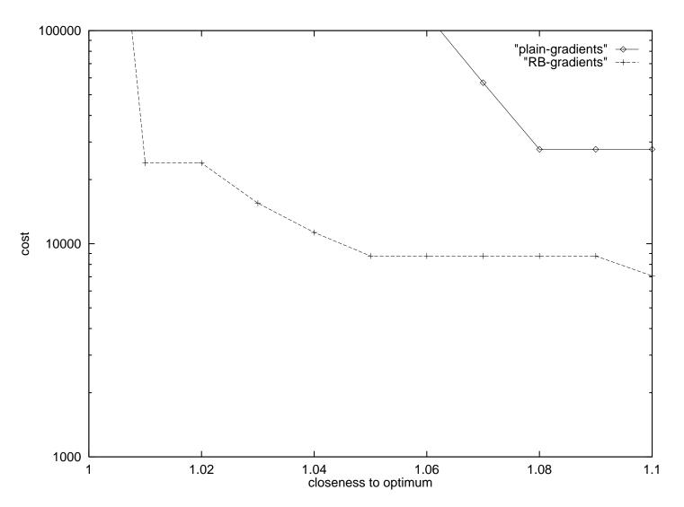
Figure 6: Performance of rule-based gradients for the missile inlet domain. Optimization performance increases as one moves down (lower cost) and to the left (closer to optimum). The cost shown is the estimated number of simulations needed to have a 99% chance of getting within the specified fraction of the optimum.
