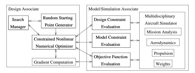
Figure 3: Automated design system block diagram
