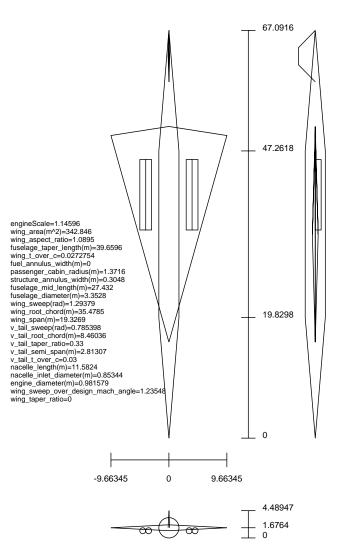
Figure 2: Supersonic transport aircraft designed by our system (dimensions in meters)
