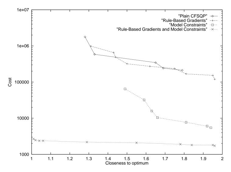
Figure 5: Performance of the various strategies for a different mission. Optimization performance increases as one moves down (lower cost) and to the left (closer to optimum). The cost shown is the estimated number of simulations needed to have a 99% chance of getting within the specified fraction of the optimum.
