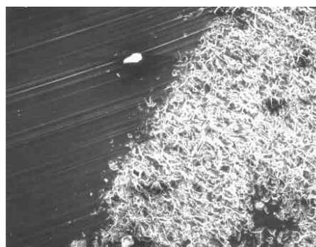
FIGURE 7(A) LEADING EDGE OF PLASTICALLY WORKED AREA OF AL FILM AFTER 3 MINUTES OF POLISHING  $\text{CaF}_2$  WITH 45  $\mu\text{m}$  DIA., 28 CM/S, 1 G/MM<sup>2</sup>, 20KV, 102X.
