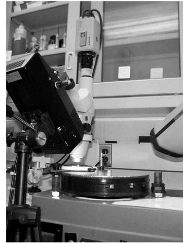
FIGURE 5(B) EXPERIMENTAL RIG USED WITH DUAL STROBE SET-UP W/REFLECTIVE TAPE ON LAP O.D. FOR STROBE TRIGGERING.
