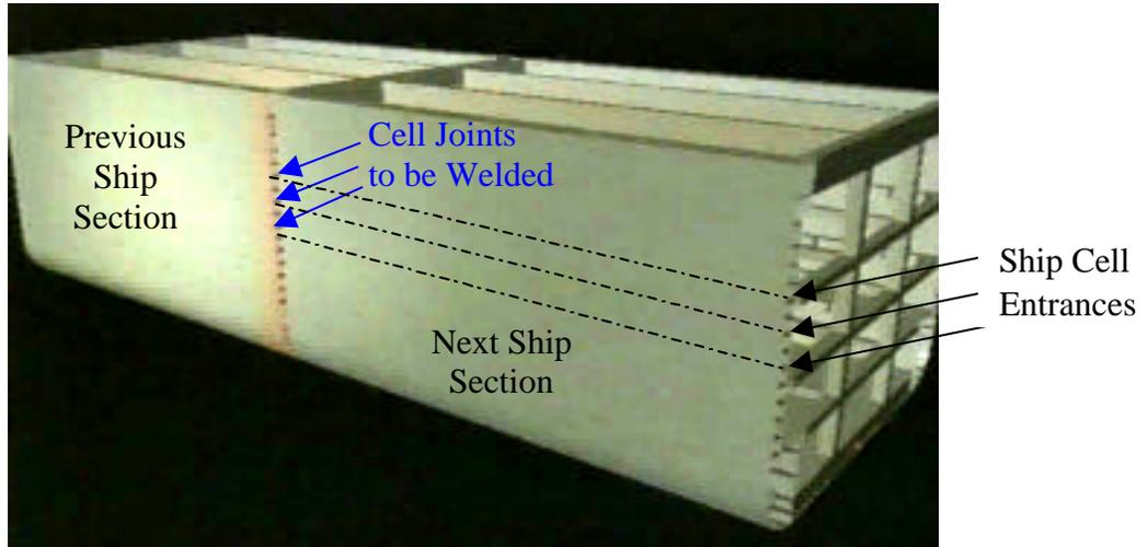
The mock-up used for the Phase 1 study was the non-combatant ship-cell size fabricated from 19 mm (0.75 in) thick steel. It measured 1.2 m wide x 1.2 m high x 2.4 m long (4 ft x 4 ft x 8 ft long) with a cell entrance measuring 0.46 m wide x 0.76 m high (18 in x 30 in). Three main components were needed to accomplish the remote and autonomous double hull ship welding
