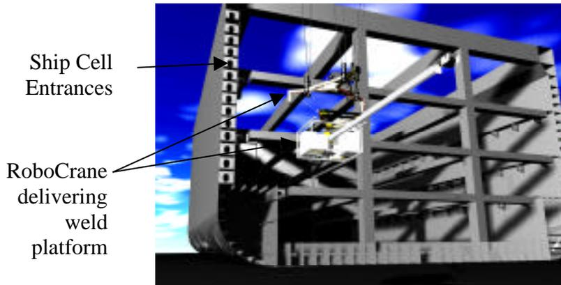
The 975 kg (2150 Lb.) weld platform, measuring 1.6 m x 1.6 m x 1.3 m high (66 in x 66 in x 53 in high), was attached to the cell mock-up during demonstration. The weld platform included static and dynamic cell attachment mechanisms, a weld torch and power supply, a robot arm and controller used to position the weld torch, a 3.7 m (12 ft) long extendable boom used to position
