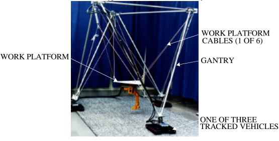
The RoboCrane's octahedron structure can be made extremely lightweight compared to conventional gantry structures.
