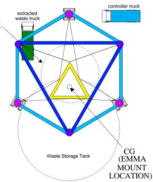
tion. Waterjet or other tools will be used to extract and retrieve the waste. The waste is pumped into a waste truck or above ground holding tank.
