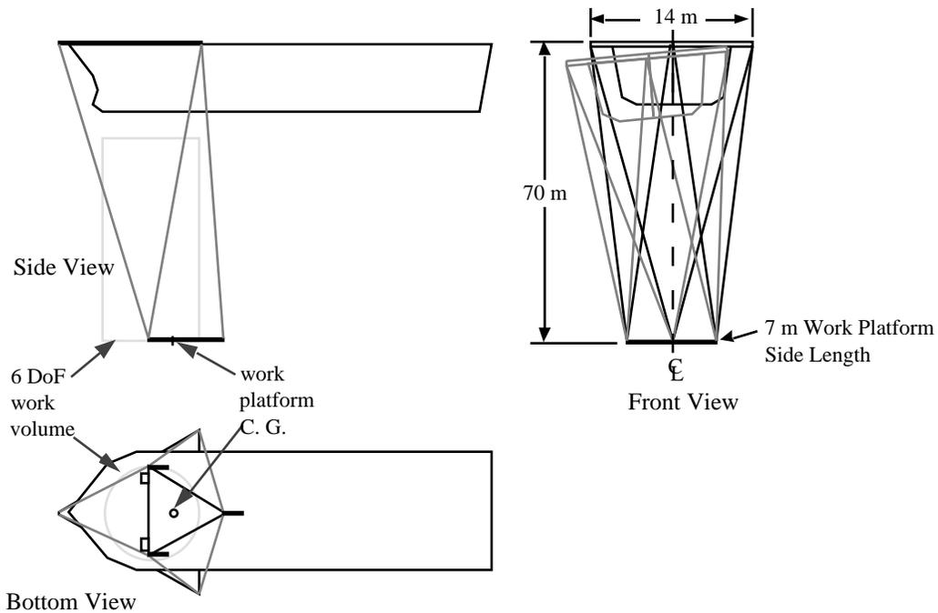
Figure 2 - Multiple views of the S3P suspended from a vessel. Front view shows orbital vessel motion with stable work platform. Side and Bottom views also show 6 DoF work volume that the work platform center-of-gravity (C.G.) can reach.
