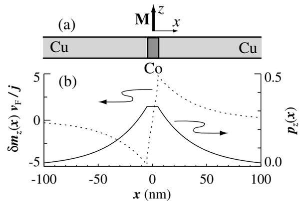
FIG. 2: Current polarization for a single ferromagnetic layer. Panel (a): a thin Co layer embedded between two semi-infinite Cu leads. Panel (b): current polarization (solid line) and spin accumulation (dotted line) for a single Co layer embedded in Cu. The spin accumulation, defined as a density rather than a magnetization, is put in a dimensionless, scaled form by dividing by the ratio of the current to the Fermi velocity.
