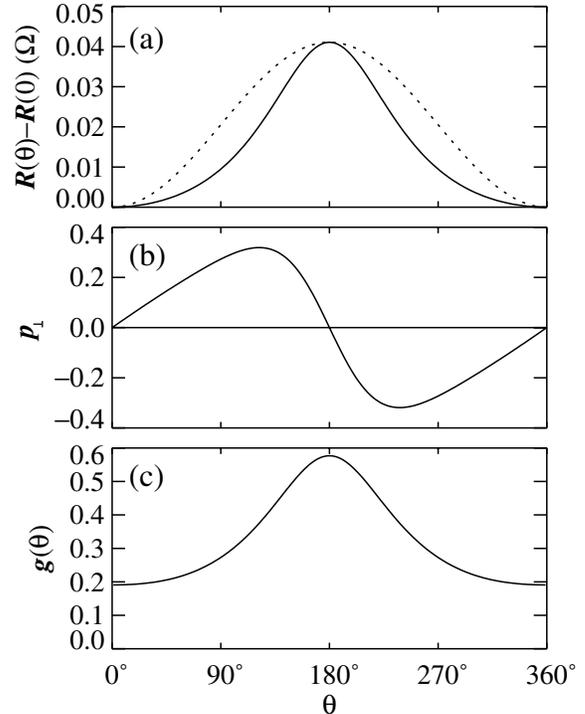
FIG. 4: Magnetoconductance and torque. Panel (a) shows the change in resistance as a function of the relative angle between the two magnetizations (solid curve). The dotted curve is proportional to  $1 - \cos \theta$ . The resistance has been computed from the values in the text and a cross-sectional area of  $\pi 65^2 \text{ nm}^2$ . Panel (b) shows the transverse current polarization on the right ferromagnetic layer. Panel (c) shows the same quantity divided by  $-\sin \theta$ .
