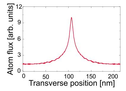
FIG. 1. Laser-focused chromium flux calculated within a semiclassical approximation by tracing trajectories of  $10^5$  atoms exiting an oven at 1900 K and collimated to a FWHM divergence of 0.16 mrad. The laser is detuned from the chromium two-level resonance by +500 MHz. A laser power of 20 mW is used, as this gives the best focusing, given the Gaussian laser  $1/e^2$  radius of 60  $\mu$ m.
