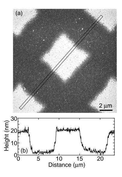
Fig. 2. (a) Tapping mode AFM image of hydrogen-passivated Si(100) following exposure to  $\sim 1 \times 10^{16} \text{ Ar}(^{3}\text{P}_{0,2})$  atoms cm<sup>-2</sup> in the presence of  $\sim 3 \times 10^{-5}$  Pa (2 × 10<sup>-7</sup> Torr) partial pressure of O<sub>2</sub> and KOH etch. (b) Section from (a) to show feature depths averaged over region indicated in box.
