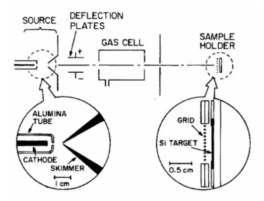
Fig. 1. Schematic of the apparatus. A beam of metastable Ar atoms, produced in a DC discharge, strikes a hydrogen-passivated Si wafer. Deflector plates remove ions and Rydberg atoms from the beam, and a gas cell provides a means to quench the metastable atoms without otherwise affecting the beam. The beam is patterned before striking the wafer by passing through a square Ni grid with 12.7  $\mu$ m pitch (5.1  $\mu$ m wires and 7.6  $\mu$ m spaces).
