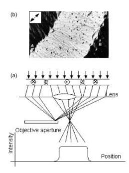
*Figure 6.15.* (a) Schematic of the Foucault or in-focus mode of domain imaging showing the use of an objective aperture to select out rays deflected in a particular direction to provide domain contrast. (b) An example a domain [also shown in Fig. 6.13(b)] as seen in the Foucault mode.<sup>50,53,57</sup>
