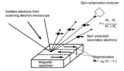
*Figure 6.1.* A schematic depiction of SEM with SEMPA apparatus. Spin-polarized secondary electrons, emitted when a finely focused incident electron beam hits the sample, are spin analyzed to determine the magnetization direction in the region under the incident beam.
