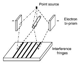
*Figure 6.18.* A schematic showing the interference resulting from electrons following paths of differing lengths from a high coherence source through the electron optical equivalent of a bi-prism. Modified from Ref. 66.
