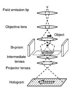
*Figure 6.20.* A schematic showing a setup for absolute holography. Here, a part of the wave passes through the object (right) and another part of it does not (left). A bi-prism is used to recombine the waves and produce an interferogram. Modified from Ref. 66.
