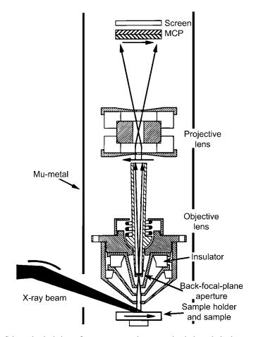
*Figure 6.23.* Schematic depiction of an apparatus that uses circularly polarized x-rays to produce secondary electrons that are then focused electrostatically to form a highly magnified image on a microchannel-plate (MCP) intensifier.<sup>79,80</sup>
