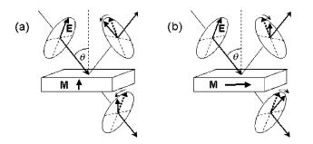
*Figure 6.8.* Light and magnetization geometries for observing the polar (a), and longitudinal (b) magnetooptic effects for either reflected or transmitted light. Modified from Ref. 2.
