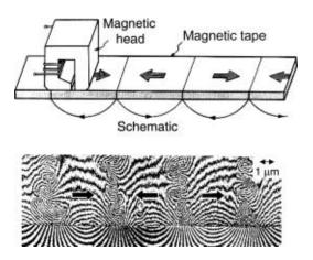
*Figure 6.21.* Top: Schematic depiction of recording method and recorded pattern. Bottom: Interference pattern revealing magnetic lines of force. The 45 nm thick Co film occupies the lower 3/4 of the image and the top 1/4 is free space. The magnetic lines of force are seen to lie along the magnetization direction within the Co and as a fringe field extending past the edge of the film. Modified from Ref. 67.
