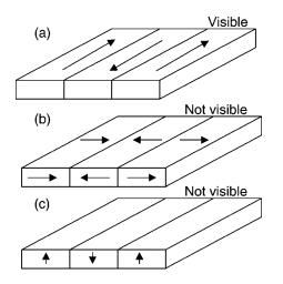
*Figure 6.14.* Three possible domain geometries, which will lead to observable (a) or non-observable (b,c) domain walls by using the Fresnel mode. Modified from Ref. 2.
