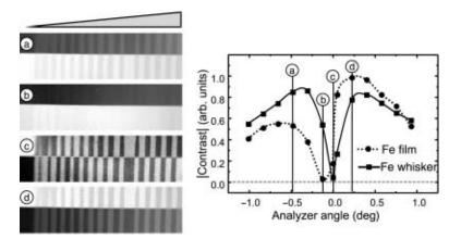
*Figure 6.12.* (a–d) Magneto-optic images of an (Fe whisker)/(Cr wedge)/(Fe film) structure as the analyzer is rotated. Magnetic contrast from the top film is extinguished in image (b), whereas the Fe whisker contrast is extinguished in (c). The absolute value of the contrast is shown in the adjoining plot.
