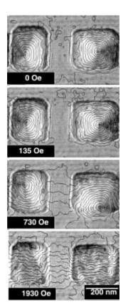
*Figure 6.22.* Holographic determination of magnetic lines of flux in Co rectangles of different shape for four values of an external magnetic field. Note how the two field distributions make a transition from a solenoidal configuration at zero applied field to a near-saturated configuration at 1930 Oe.<sup>72,73</sup>
