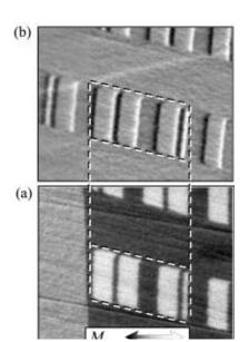
*Figure 6.6.* (a) A SEMPA image showing the  $M_x$  component of the magnetization of a high density bit pattern written on a hard magnetic disk. (b) Same structure shown in (a) as imaged using MFM. An Au mask, which can be seen in (a), covers the left-hand side of the sample. From Ref. 27.
