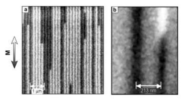
*Figure 6.5.* (a) SEMPA image of an array of Fe nanowires showing their in-plane magnetization,  $M_y$ , where white (black) indicates up (down). (b) A high-resolution SEMPA image showing a domain wall within a wire. From Ref. 21.
