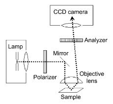
*Figure 6.9.* A schematic of a magneto-optical microscope for high-resolution imaging of magnetic microstructure in the longitudinal Kerr mode. Modified from Ref. 2.
