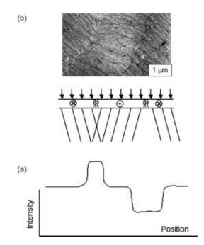
*Figure 6.13.* (a) Schematic depiction of deflection of defocused incident electron beam upon transmission through a thin magnetic sample illustrating the formation of bright and dark, domain wall structures. (b) Example of two domain walls, white (A) and black (B), in a thin film  $Fe_{81}B_{13.5}Si_{3.5}C_2$  sample.<sup>57</sup>
