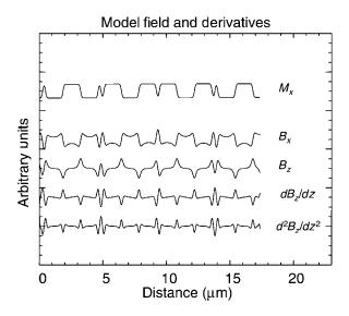
Figure 6.7. A magnetization distribution modeled after the SEMPA measurements shown in Fig. 6.6(a) and several fields and field gradients derived from that distribution. From Ref. 27.
