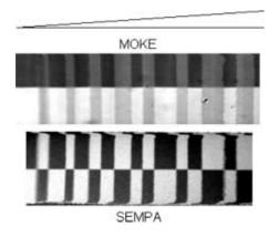
*Figure 6.11.* Magneto-optic and SEMPA images of the same multilayer structure. The difference in the appearance between the two images is due to the different probing depths of the two methods. The sample consists of an Fe whisker substrate, 0–23 layer Au wedge, 12 layers of Fe, and six Au layer overcoat. Modified from Ref. 20.
