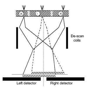
*Figure 6.17.* A schematic depiction of the DPC mode of imaging in which split detectors are used to monitor the angular deflections that electrons incur on transmission through ferromagnetic domains.<sup>52,65</sup>
