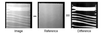
*Figure 6.10.* An example of digital image subtraction to reduce the non-magnetic background signal in a longitudinal Kerr image. A reference image of the Permalloy rectangle, acquired in a magnetic field large enough to saturate the magnetization, was subtracted from an image acquired at zero applied field.
