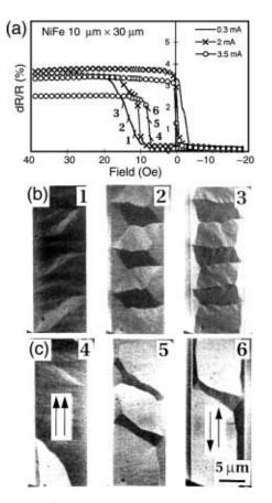
*Figure 6.16.* (a) GMR curves of a NiFe spin valve measured *in situ* during Foucault mode domain observations shown in (b) and (c). Three different currents were applied to the device to measure the GMR. (b), (c) Domain images of the spin valve corresponding to the measurement points indicated in (a) for applied currents of 0.3 and 3.5 mA, respectively.<sup>58,59</sup>
