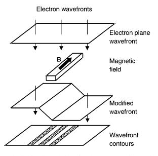
*Figure 6.19.* A schematic showing the evolution of a plane wave wavefront as it passes a magnetic material. Modified from Ref. 66.
