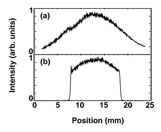
FIG. 2. Laser intensity profiles along the direction of the atom beam, measured at the interaction region: (a) full Gaussian profile and (b) truncated profile. A fit to the Gaussian profile yields a  $1/e^2$  full width of  $23 \pm 1$  mm. The truncated profile has a full-width at half-maximum of  $10.6 \pm 0.5$  mm. The laser profile perpendicular to the atom beam (not shown) was very nearly Gaussian with  $1/e^2$  full width of  $4.2 \pm 0.2$  mm.
