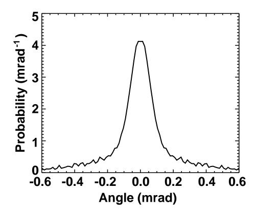
FIG. 4. Angular distribution of the cooled Cr beam obtained by inverting and symmetrizing a derivative profile such as shown in Fig. 3b. This distribution corresponds to the highest degree of collimation observed, obtained by using a Gaussian laser beam (Fig. 2a) with total power 40 mW and detuning  $-\Gamma$ . 90% of the atoms are within 0.61 ± 0.02 mrad and 50% are within 0.16 ± 0.01 mrad.
