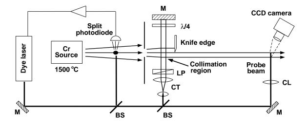
FIG. 1. Experimental arrangement, showing effusive chromium source (at 1550 °C) with 1 mm diameter aperture, split photodiode for frequency locking, precollimating aperture  $(1 \text{ mm} \times 1 \text{ mm})$ , molasses region, knife edge and fluorescence imaging detector. The optical elements shown are mirror (M), beamsplitter (BS), linear polarizer (LP), cylindrical telescope (CT), cylindrical lens (CL) and quarter-wave retarder ( $\lambda/4$ ).
