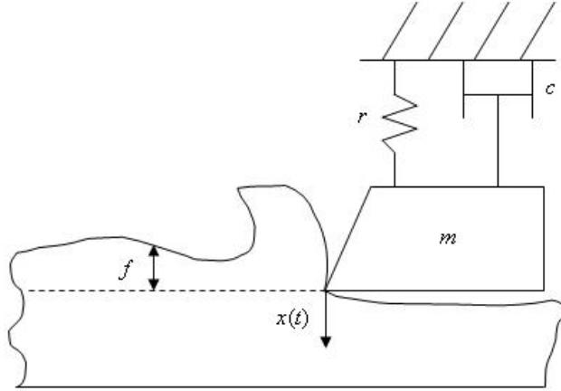
**Fig. 3.** One Degree-of-Freedom-Model for Single-Point Turning
