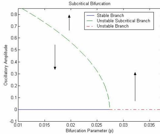
**Fig. 6.** Amplitudes of Bifurcating Branches of Solutions at Subcritical Point
